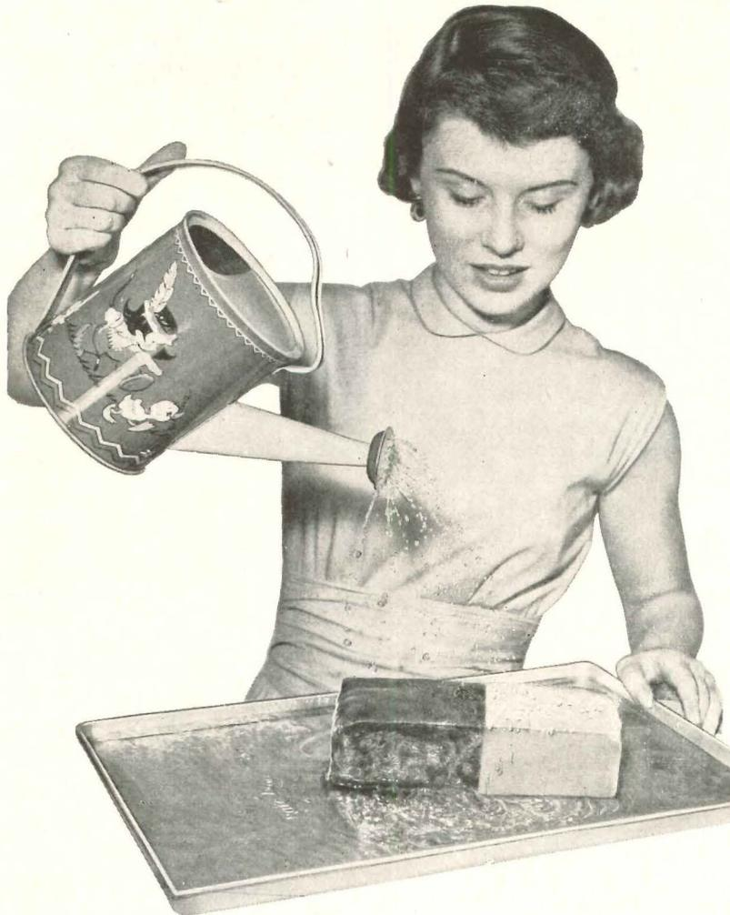
Note how water refuses to penetrate right half of masonry block (treated with G-E silicone water repellent) while untreated left half is saturated.
