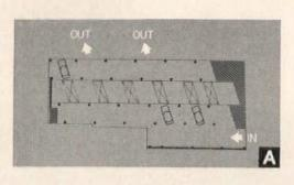
The 12-level scheme designed by Friedman, Alschuler and Sincere, Architects (right and above) will accommodate 495 cars and is intended primarily for short time parkers. The hoist shaft, separating entrances and exits, will be brick sheathed, with granite faced lobby. Open floor slabs of architectural concrete will have aluminum guard rails
