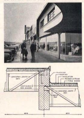
Typical section of through party wall between stores of different ceiling height.
