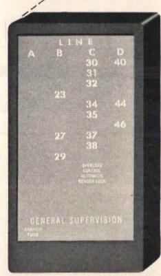
Signal control panel, monitoring 4 lines shows that Line "A" is inoperative due to blown "Branch Fuse." Lines "B" and "D" signal that carriers are on the way to stations 23, 27, 29, 40, 44 and 46. In Line C the "Overload Control Automatic Sender Lock" has closed the line to additional carriers until a momentary congestion lessens. Meanwhile carriers proceed to stations 30, 31, 32, 34, 35, 37 and 38.
