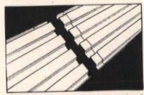
Ends of Robertson Q-Deck are sized and countersunk to produce a tight, smooth, two-inch lap joint. This lap, along with the tight side laps, provides a vaporsealed roof construction.
