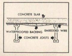
NOTE: In the cross section that the weight of the wet concrete forces the backing away, which permits the galvanized steel mesh to assume its proper position in the slab. Steeltex floor lath also performs two other functions: It permits work on the floor below while pouring is in progress and retains moisture to assist proper curing.
