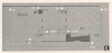
Capable of accommodating 665 cars, the ramptype garage designed by Everett F. Quinn and Associates, Architects (below and left) is a splitlevel scheme four stories in height. The granite and face brick treatment at the entrances contrasts with the perimeter concrete guard rails at the various levels
