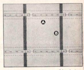
Supporting splines (A) are parallel to furring, and continue through tile joints. Fiber cross splines (B) are used for leveling. They are not stapled, making installation still more economical.
