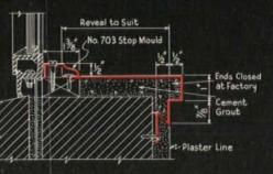
Cross-section shows No. 521 installed where flat window stool is desired. Cement grouting is recommended for good construction.
