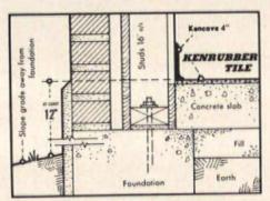
Above diagram shows approved installation of KenRubber over concrete in contact with the earth.
