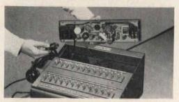
"Inside Story" . . Plug-in connections allow built-in amplifier to be removed easily for service. Tubes replaced by simply removing screen ventilating grill at rear of cabinet.
