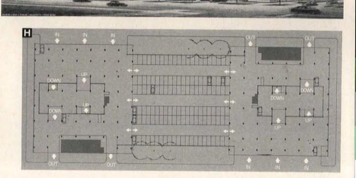
Unusual solution by Architects Holabird and Root and Burgee (plan and rendering above) consists of two buildings bounding a central parking lot enclosed by two serpentine walls
