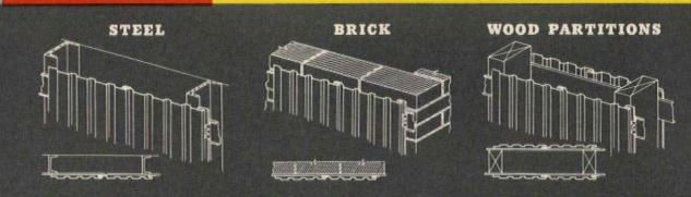
Application of Zourite to steel, masonry or wood construction is quick and simple with the patented Anchor Clip and Zourite Furring Channel spaced 24" O.C. It's lightweight and is easily cut on the job or shop fabricated. Zourite is made of .050 thick aluminum and is available in 4 widths from 2½" to 8½" and there are 9 trim members to meet all corner and edge conditions. Phone, wire or write now for additional technical information.
