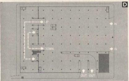
A ramp-type structure for 1000 cars, the garage designed by Schmidt, Garden and Erickson, Architects (above and left) consists of five split levels. The horizontal treatment is emphasized by the concrete and aluminum guard rails; entrances are of face brick. Intensity of perimeter lighting automatically controlled photo-electrically
