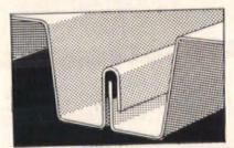
Robertson Q-Deck side laps are designed to form a standing seam. A seal in the form of a continuous caulking material assures a vapor-tight joint.
