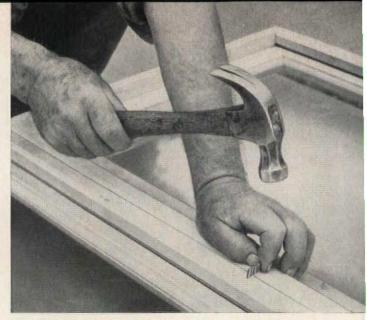
"Versatile Andersen Flexivents," reports Hilferding, "make it possible to offer customers a wide selection with moderate inventory." Here, a shop workman places Flexivents in position for joining, Joining with corrugated fasteners is the best.
