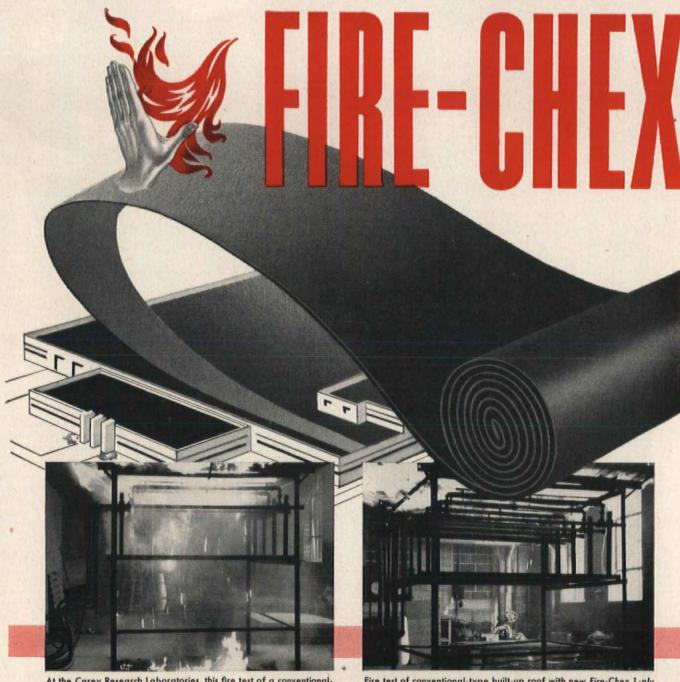
At the Carey Research Laboratories, this fire test of a conventionalvapor seal, with insulation and built-up roofing over steel deck, showed the dripping of asphalt from the vapor seal igniting as 1800° of heat builds up under the roof construction and melted bitumen flows through the joints in the deck.
