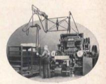
BESSER VIBRAPAC - the fully outematic concrete block machine. Produces high quality masonry units, of any desired texture and density, at the lowest possible cost. A 7737-1PB
