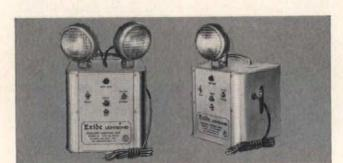
THE NEW MODEL M has a two-rate charger—high rate or trickle. After the emergency, automatic controls recharge the Exide battery specially developed for dependable operation, long life, less maintenance. UL-approved. Plugs into any 115 volt outlet. Single and double lamp units are available; each lamp illuminates up to 10,000 sq. ft.
