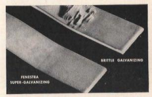
BEND TEST shows why Fenestra Steel Windows are called Super Hot-Dip Galvanized. When two pieces of galvanized steel are bent, then straightened, some types of galvanizing crack open, leaving the steel vulnerable. The Fenestra piece stays protected.
