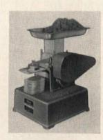
32. The Hollymatic Corp. patty-molding machine makes round, square or chop-shape patties in any thickness. Said to produce 2100 patties an hour, the molder is completely automatic, eliminating time-consuming manual paper feeding. (433 W. 83 St., Chicago, III.)
