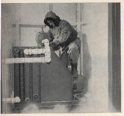
Cold as Siberia—or the stratosphere! This room, capable of creating 65-degrees-below-zero cold, is designed for testing the performance of Trank equipment at low temperatures. Here, a radar tube cooler test set-up is being checked under conditions it might face in some bitterly cold Arctic plane-spotting station.
