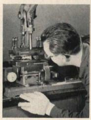
The ability of Kentile's top-grade raw materials to flow properly during calendering is measured by a Mooney Viscometer.
