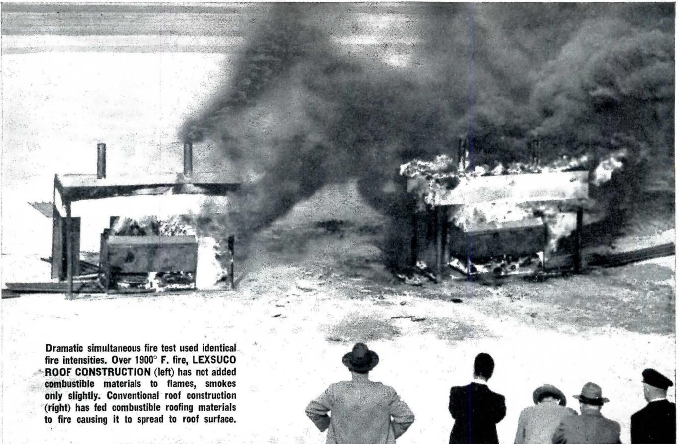
Dramatic simultaneous fire test used identical fire intensities. Over 1900° F. fire, LEXSUCO ROOF CONSTRUCTION (left) has not added combustible materials to flames, smokes only slightly. Conventional roof construction (right) has fed combustible roofing materials to fire causing it to spread to roof surface.
