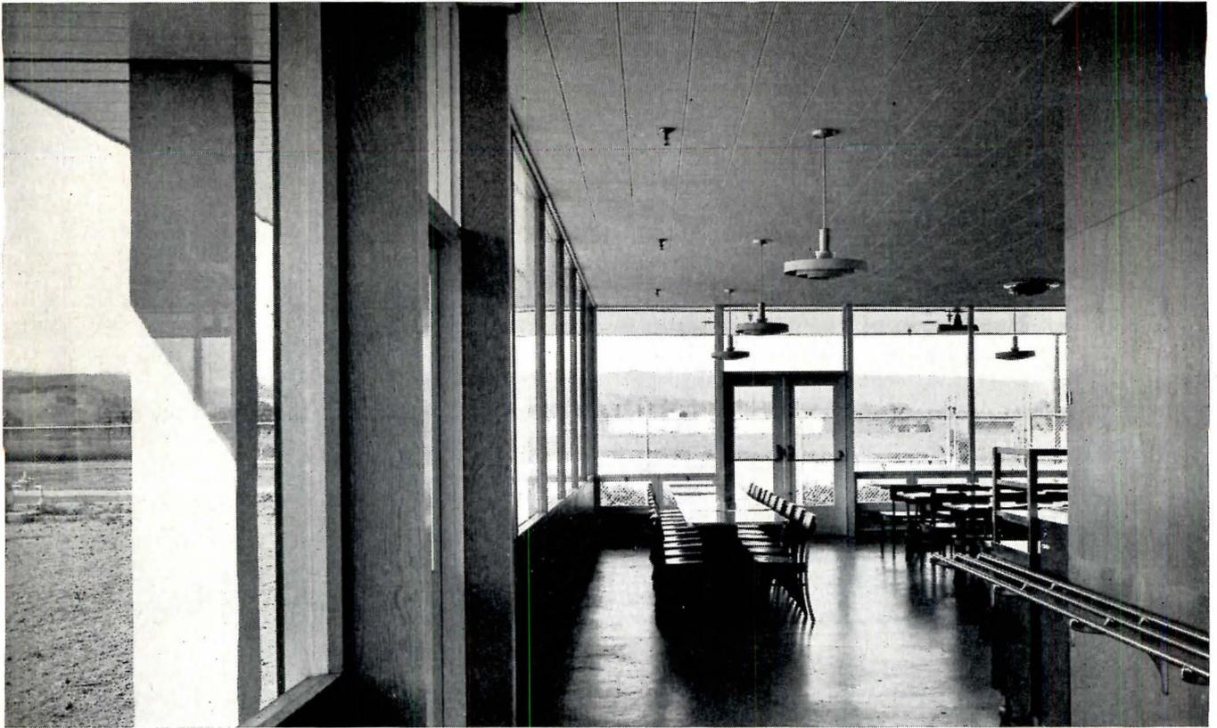
Except for the concrete columns the building is of wood frame construction. Column spacing varies from 20 to 24 ft. Roof trusses, however, are not carried directly by these columns; they rest on steel beams which run the length of the wings (see detail). Truss spacing is 7 ft 6 in. The wood construction required sprinkler protection throughout, including attic, open corridor and covered walkway.
