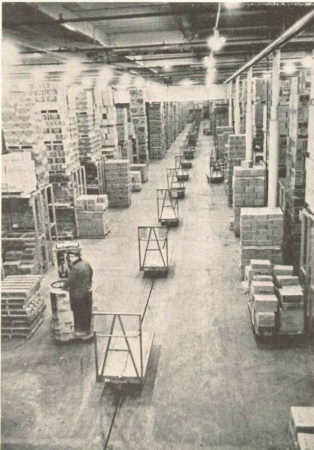
THE FIRST MODERN one-story "streamliner" food distribution depots were built in the early 1930's. They had 14 ft. ceilings. Their operators put cubage to use and handled tonnage on skids and high-lift platform trucks. What was then called the assembly line was in use, though still controversial.
