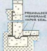
The proper installation of Premoulded Membrane to the exterior of the basement walls as well as beneath the floor slab insures a permanently warm and dry basement.
