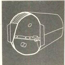
**Adequate Venting** Venting should be suited to the function: for exhaust of heat, fire, smoke or gases or for release of explosion pressures
