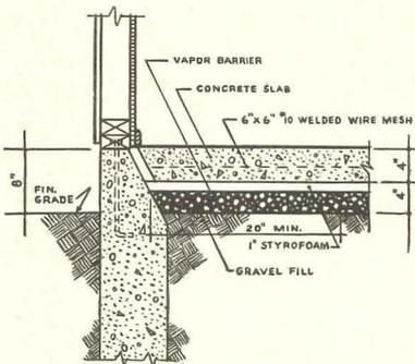
Styrofoam used in a horizontal position for perimeter insulation. One to two inches of Styrofoam is used for a distance of 12"-24" in from perimeter, meeting F.H.A. minimum requirements in various climatic areas. Due to the strength and moisture resistance of Styrofoam, the concrete floor can be poured directly over it without compressing the Styrofoam.
