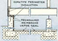
The proper installation of Premoulded Membrane and Corkite removes all danger of condensation and oxidation of metal installations in the crawl space area... eliminates the need for ventilation.
