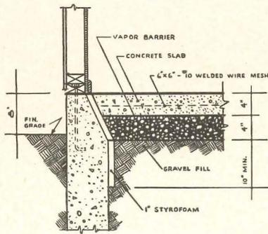
Styrofoam is being used in a vertical position for perimeter insulation. It can be adhered in place or held by back fill. Minimum F.H.A. requirements in vertical position are one to two inches thick from floor line to a depth of 12"-24" below grade line depending on climatic conditions.
