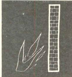
**Protected Steel Members** *Steel members will expand and buckle under heat of sufficient intensity, and so they should be protected with a fire-resistive covering*
