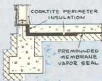
This illustration shows how the installation of Premoulded Membrane and Corkite completely isolates the slab and superstructure from soil moisture.
