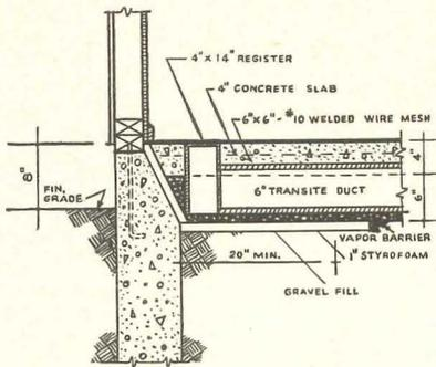
In this perimeter heating application, Styrofoam is used both vertically above grade and horizontally from outer edge of slab on the grade. One inch thick Styrofoam perimeter insulation in a 1'-1½' combined vertical and horizontal width is accepted by F.H.A. for perimeter, radial and radiant type slab heating systems.
