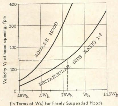
several curves on each of the graphs. These curves are labeled for different side ratios (hood width: hood length). A control velocity  $V_c$  of 30 fpm was used in calculation of these curves. Knowing the side ratio, hood width and distance  $X$ , the face velocity  $V_f$  can be found from the curves and the hood exhaust volume calculated using the formula  $Q = V_f \times A_h$ .
