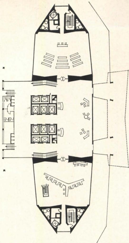
The plans make clear the manner in which the bifurcated columns diminish in area towards the building's summit. In the small plan, left page, C indicates the truck entrance and lift; D shows the glass-enclosed gallery where visitors may view mechanical and electrical equipment, located in the area noted as B
