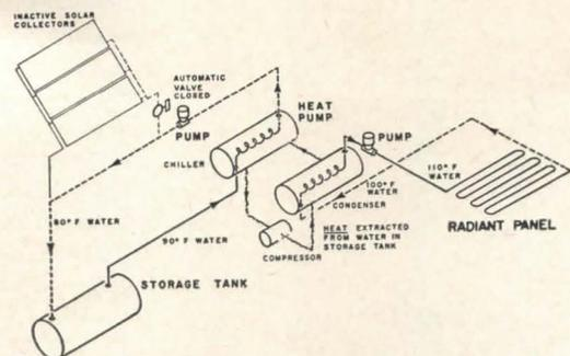
During extended dark days, heat pump heats building. Heat pump can also be used for summer cooling, with cooled water from chiller going directly into radiant system and extracted heat being discharged to the outside through evaporative water cooler
