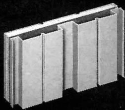
**NEW Fenestra Type "FA" Wall Panel** — Designed for simple, fast field assembly. Distinctive exterior design with deeply revealed fluting. Exterior — galvanized steel or grained aluminum (porcelain enamel optional). Interior — galvanized steel. Width 24". Lengths to 31'. Depth 3".
