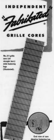
These grille cores are used for openings in pre-fabricated partitions, room cooling cabinets, radiator tops, etc. Furnished to order, such cores can be supplied in practically any overall size. Mesh openings are standard %" x 11%" and cannot be varied.
