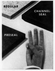
A type for every job requirement. PRESEAL: Asphalt-coated on both faces and edges for greater protection against moisture pick-up. CHANNEL-SEAL: Bevels on deck-side form network of channels for equalization of air and vapor pressure, providing extra protection against blistering and separation of felt and insulation, asphalt-coated. REGULAR: Uncoated Celotex board. Recognized standard where lowest cost insulation is required. All in a variety of thicknesses.
