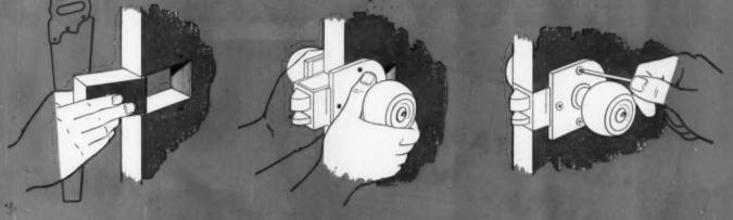
Make a simple cut-out and two bolt holes in the door, slip the lock into place, apply through bolts and tighten. That's how easy it is to install a CORBIN Unit Lock ... any one of the 20 available functions! Unit Locks are the only type locks completely assembled at the factory with knobs and escutcheons attached. There's nothing to take apart and reassemble ... practically no chance of misapplications!
