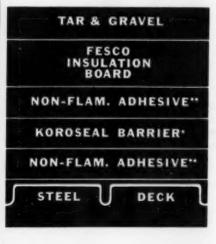
In every way, Fesco Board lent itself to a new concept in fire retardant roof design employed on the 34 acre roof of Chrysler's Twinsburg, Ohio body stamping plant. Teamed up with Lexsuco's non-flammable adhesive, and the modern vapor barrier, Koroseal\*, Fesco Board contributed these important properties:
