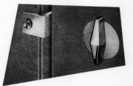
SEEN FROM INSIDE OF COMPARTMENT – latch presents smooth flush lines and minimum projections. Latch handle operates with smooth cam action, has no springs; (tested to 300,000 cycles of operation without noticeable wear).
