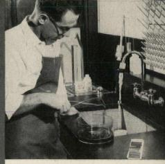
3 Cleaning specimens with inhibited hydrochloric acid
