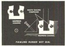
"Wet" seal combines pressure seal with twosided adhesive seal. A reservoir of mastic
