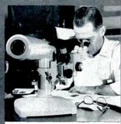
Final examination of specimens under low power magnification
