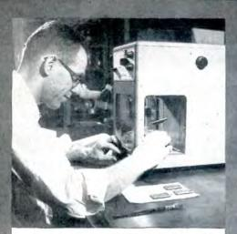
1 Analytical weighing of specimens prior to testing
