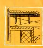
Typical detail and photo of Kalser Aluminum's Type K-1 Gravel Stop. Note simplicity and pleasing shadow line that results from the straight drip edge feature.
