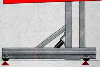
With no spectator load on seats, roller housings and uprights are raised leaving casters "free" for smooth, easy operation.
