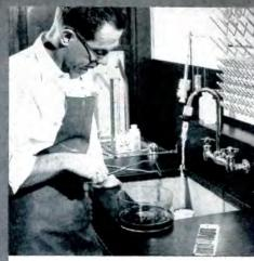
3 Cleaning specimens with inhibited hydrochloric acid
