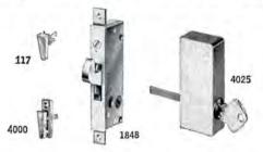
The 1848 Sliding Wall Deadlock shown above measures only  $3\%'' \times 1\%'' \times 1/2''$ , has a collapsible bolt for protection of door and lock, and operates with positive "feel appeal". To compensate for possible misalignment of door and jamb, bolt projection can be adjusted a full 3%'' by simply turning a screw in the lock face. The 4025 cylinder group is a clean-lined outside pull, offering key control that can be keyed-in with most popular cylinder systems.
