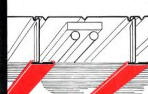
Spans up to 32 feet. Available in  $4\frac{1}{2}$ ", 6" and  $7\frac{1}{2}$ " depths; 14, 16 and 18 gauges.
