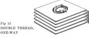
Ramps are steeper since they only have 180 deg to get between floors. A popular design with separated flow
