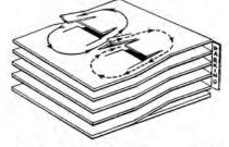
In this arrangement, the circulation has been completely separated. This is the most straightforward of the staggered floor systems
