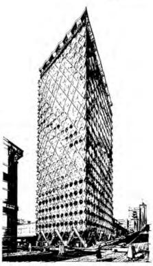
First solution—space frame 22 stories high with hexagonal windows resulting from stress pattern—was set aside when program conditions changed
