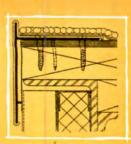
Typical detail and photo of Kaiser Aluminum's Type K-1 Gravel Stop. Note simplicity and pleasing shadow line that results from the straight drip edge feature.
