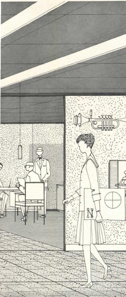
**JOHNS-MANVILLE MOVABLE WALLS** provide architects with modular components that are functional and attractive in appearance for the design of space-division layouts. They can be erected, dismantled and relocated over and over again.
