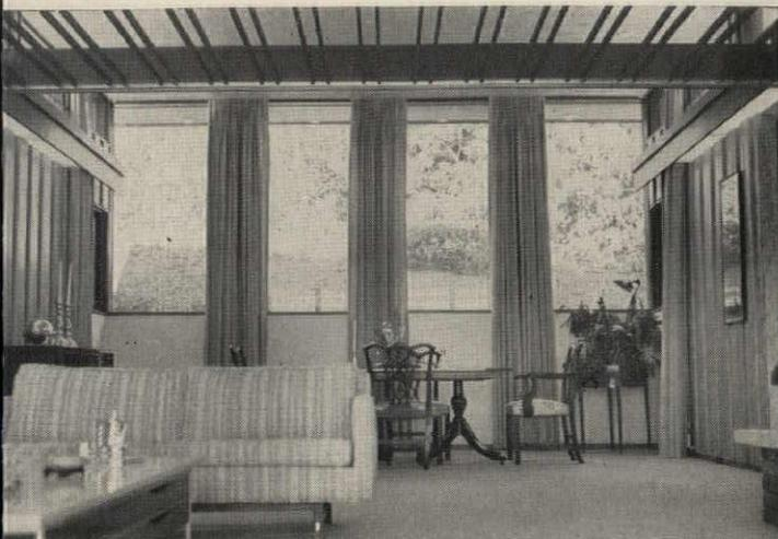
VOLK RESIDENCE, Smoke Rise, N. J. All exterior window walls were constructed of shop-built, prefabricated modular frames, all dimensioned around standard *Thermopane* sizes. These same panel types, which were fitted into the modular wood framing system, together forming the structural wall and exterior and interior finish, accommodate standard steel sash, blank opaque walls, French doors and regularly hinged doors.
