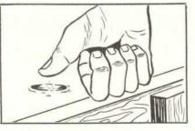
5. Give final steel troweling when thumb pressure barely dents the concrete surface.
