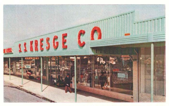
In this new shopping center, building facing, as well as canopy soffet are EGSCO Shadowall Panels. Color is baked-on epoxy enamel. Canopy facia was specially formed of the same durable metal and color.
