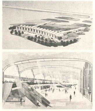
Arvin Shaw III, Carson & Lundin: 2-story concourse is daylighted by large glass areas in front and rear walls and skylights between barrel vaulted roof sections
