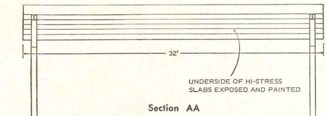
ONE-STORY COMMERCIAL BUILDING ROOF DESIGN requires only a steel frame on each side of the building to carry 8-inch Hi-Stress units on long clear span. Design can be repeated in any direction for larger building. Underside of slabs was exposed for neat, maintenance-free ceiling.
