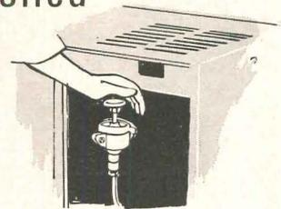
**PUSHBUTTON LUBRICATION!** An optional feature that pays for itself fast! Just push a button and metered amounts of lubricant flow to every oiling point.
