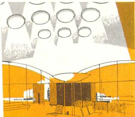
Big span of concrete shell roof permits spacious, column-free interior, with ceiling 23½ feet high at center. 21 skylights piercing the thin shell create dramatic light patterns.
