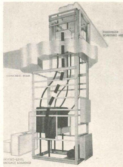
guide rails keep the car platform level while passing curves. *D. A. Matot, Inc., 1533 W. Altgeld, Chicago 14, Ill.*
