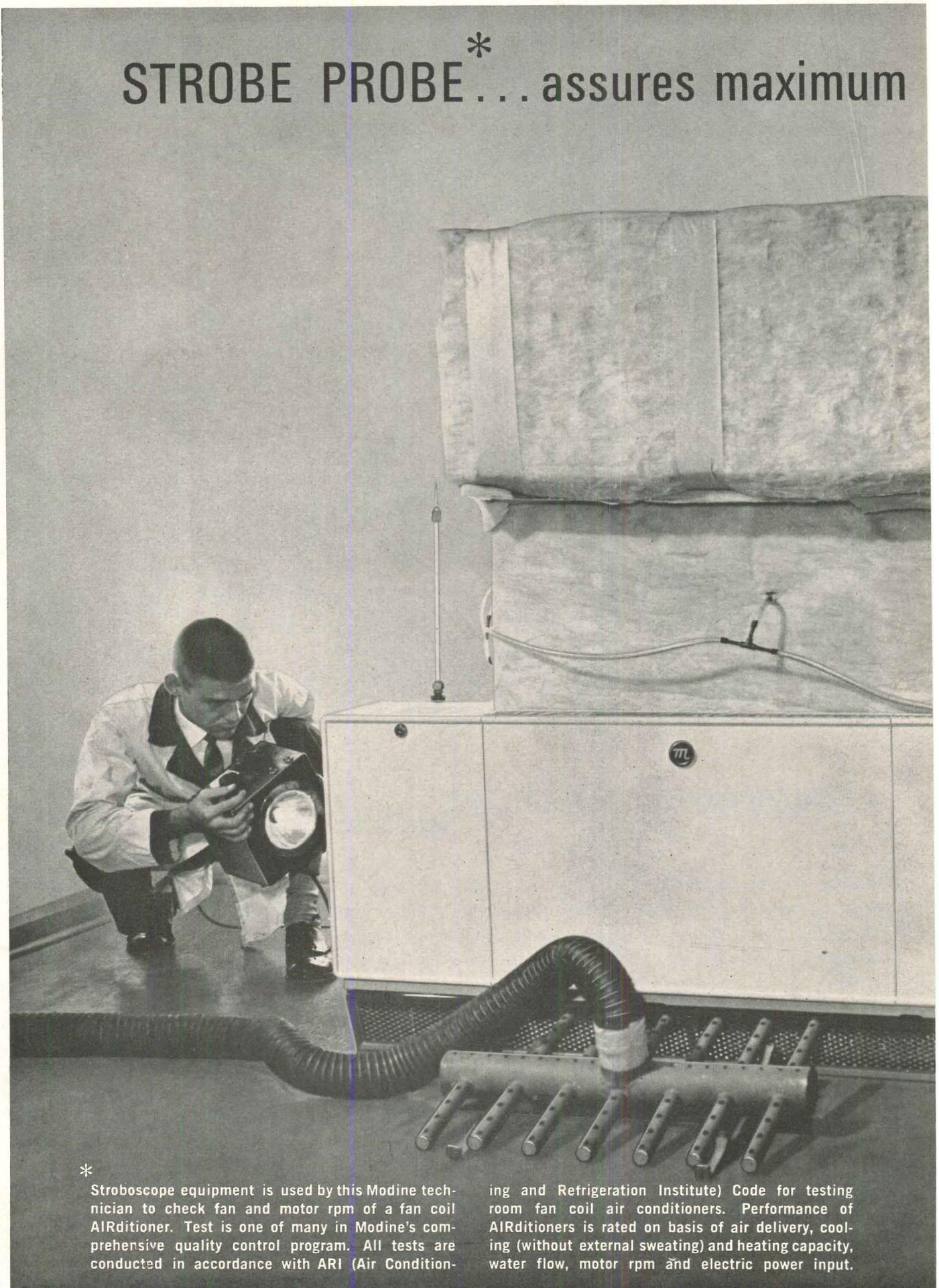
\* Stroboscope equipment is used by this Modine technician to check fan and motor rpm of a fan coil AIRditioner. Test is one of many in Modine's comprehensive quality control program. All tests are conducted in accordance with ARI (Air Condition-
