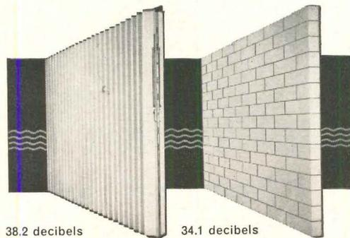
\*Geiger and Hamme Laboratory Tests (full scale) show that in a 14' x 9' opening under simulated field conditions, the average sound reduction of a Soundmaster 240 operable wall is 38.2 decibels, compared with 34.1 decibels for a 4" cinder block wall painted on both sides.
