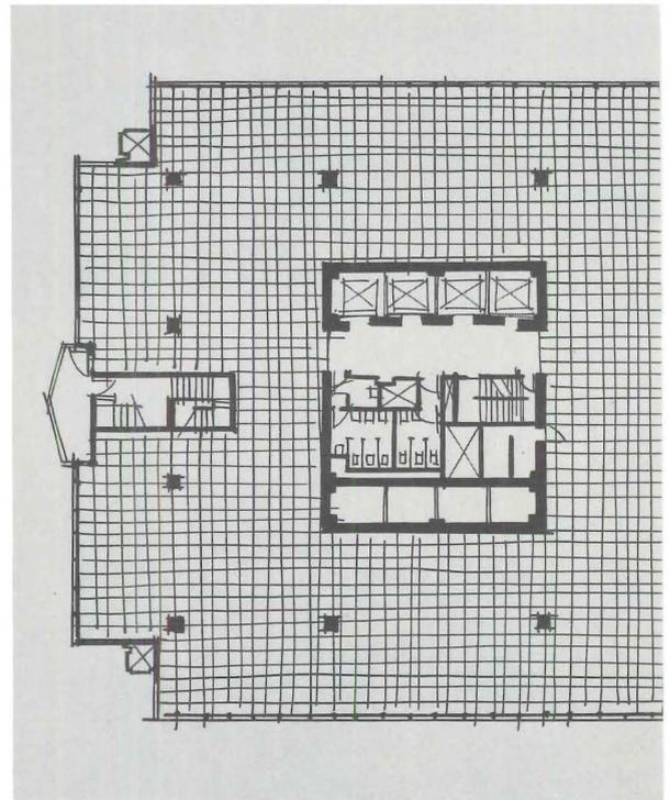
Note the corner cut-outs. This design avoided costly structural detailing and actually paid dividends by providing eight—instead of four—desirable corner offices on each floor. The architects used part of this space for air-conditioning ducts, finished in colorful porcelain-enamelled steel that enhances the beauty of the building.
