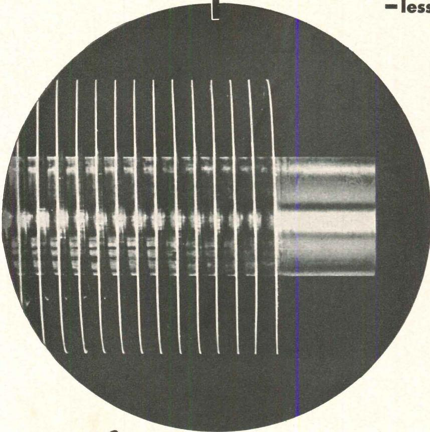
Aerofin smooth fins can be spaced as closely as 14 per inch with low air friction. Consequently, the heat-exchange capacity per square foot of face area is extremely high and the use of high air velocities highly practical. Tapered fin construction provides ample tube-contact surface so that the entire fin becomes effective transfer surface. Standardized encased units are arranged for simple, quick, economical installation.
