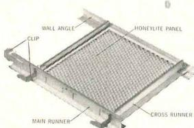
**VARIETY OF CUT-OFF ANGLES FOR SCREENING** electrical and mechanical installations in the plenum. Three cut-off angles offered: 45°, 52.5°, and 60°.
