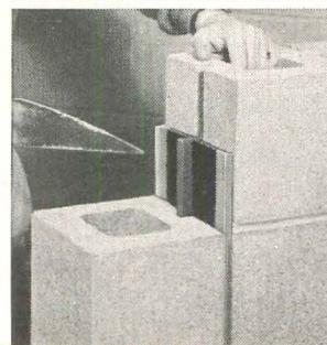
*Strength with flexibility—the two basic factors for a repair-free masonry wall are assured by these engineered companion products. Dur-o-wal reinforcement, top left, increases flexural strength 71 to 261 per cent, depending on weight Dur-o-wal, number of courses, type of mortar. The ready-made Rapid Control Joint, beneath with its neoprene compound flange flexes with the wall, keeps itself sealed tight.*
