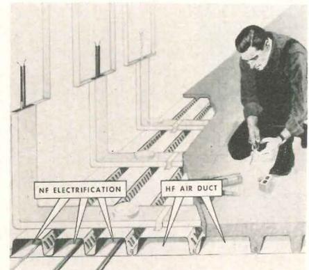
Environmental control in multi-story buildings can be achieved at low cost with an integrated air-floor system developed by Inland Steel Products Company using the products of other companies in conjunction with Inland's *Cellufloor*, a cellular steel sub-floor which carries all supply and re-
