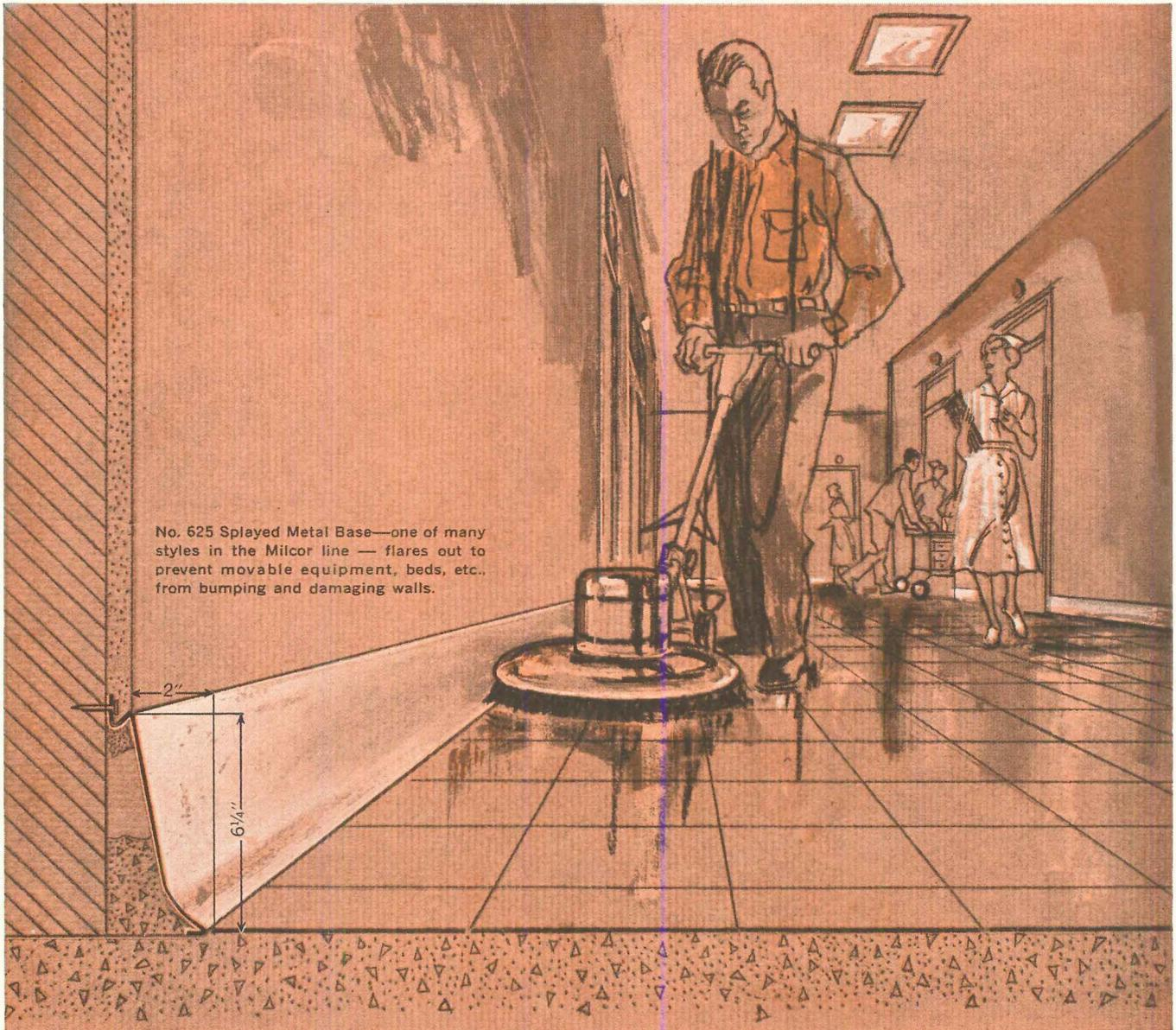
No. 625 Splayed Metal Base—one of many styles in the Milcor line — flares out to prevent movable equipment, beds, etc., from bumping and damaging walls.
