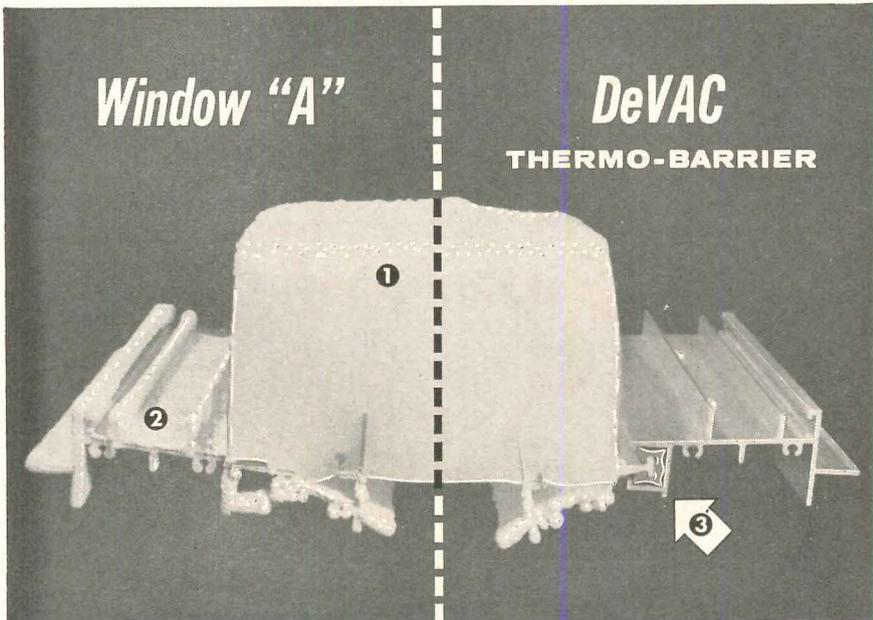
① Dry ice is used at  $-240^{\circ}$  to demonstrate conductivity of two aluminum window sections. ② Window "A" without Thermo-Barrier accumulates heavy frost and condensation. ③ Thermo-Barrier in DeVAC window halts frost and condensation, keeps inside sill dry and free of moisture.
