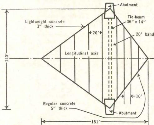
This sketch shows the “unbalanced” design of the h/p roof. Concreting sequence started with the placing of the 36" x 14" tie beam below grade. The 20' band of the shell between abutments came next. After tensioning both tie beam and 20' band, abutments were poured. Concrete for the rest of the shell was placed by alternating pours of lightweight and normal concrete. Lightweight pours were in 20' bands, normal pours in 10' bands.
