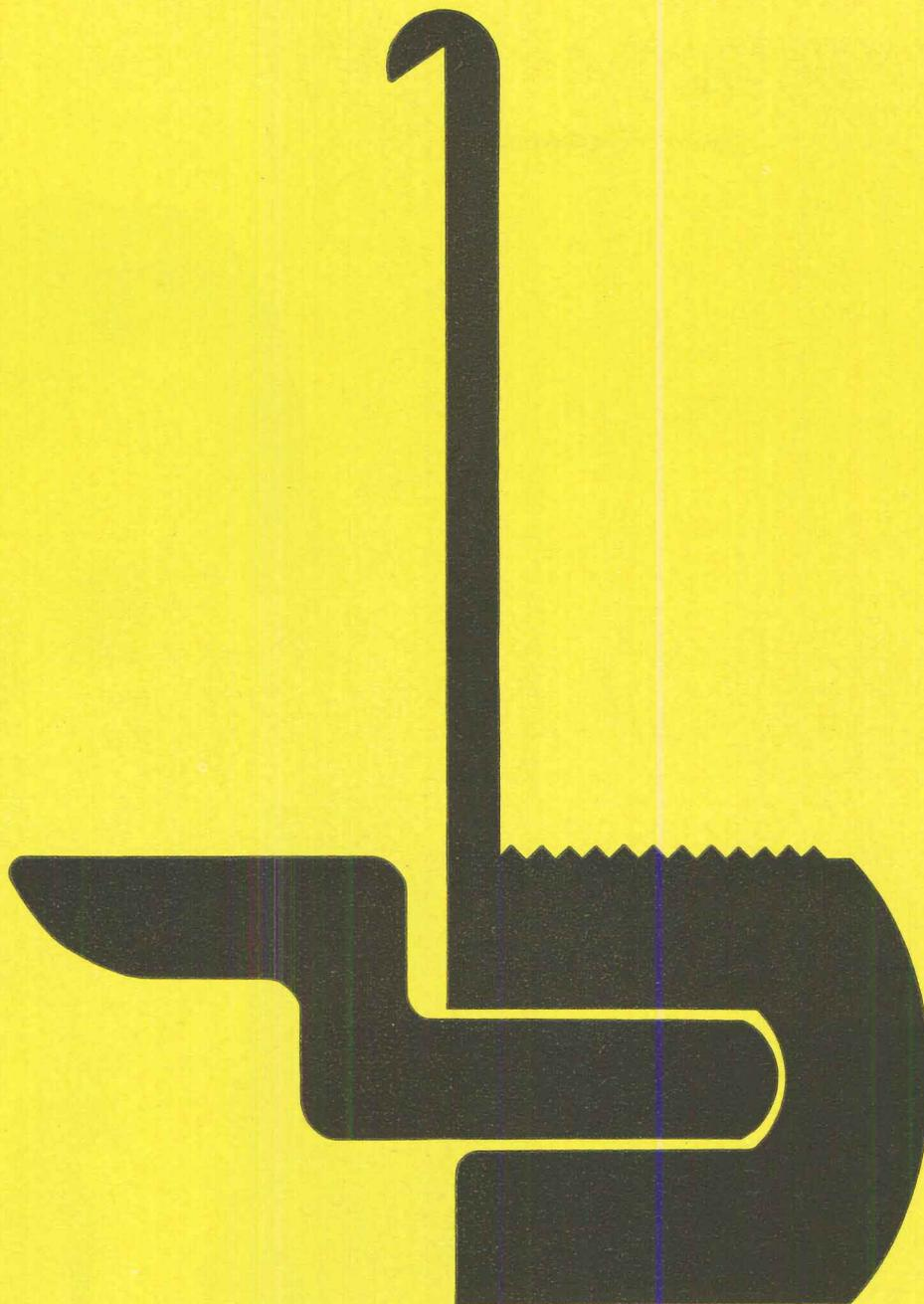
**This clamp cuts fixed window installation time by seventy-five percent. An Adlake first,\* it holds glass, weatherseal and glazing strip under proper compression. Does so automatically and never needs adjusting. Anchors the window frame to the building without a single screw. Put this clamp to work for you—and save substantially on your next stationary fenestration. Write for Bulletin 406.**
