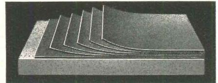
**3.** Roof is completed by building up standard roofing felts in conventional manner, either by hand or by machine.
