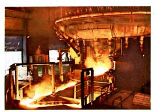
· Tapping molten iron from a blast furnace
