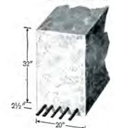
ASTM A-15 Intermediate Grade 4#11 + 1#9 As=7.24 sq. in. f'c=2500 psi fs=20,000 psi Basic Design
