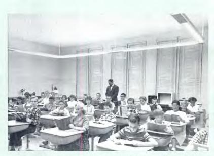
Oak St. School, Inglewood, Calif., increased light level 72%, reduced operating costs 58%, and eliminated blackboard glare by replacing incandescent fixtures with this new system.
