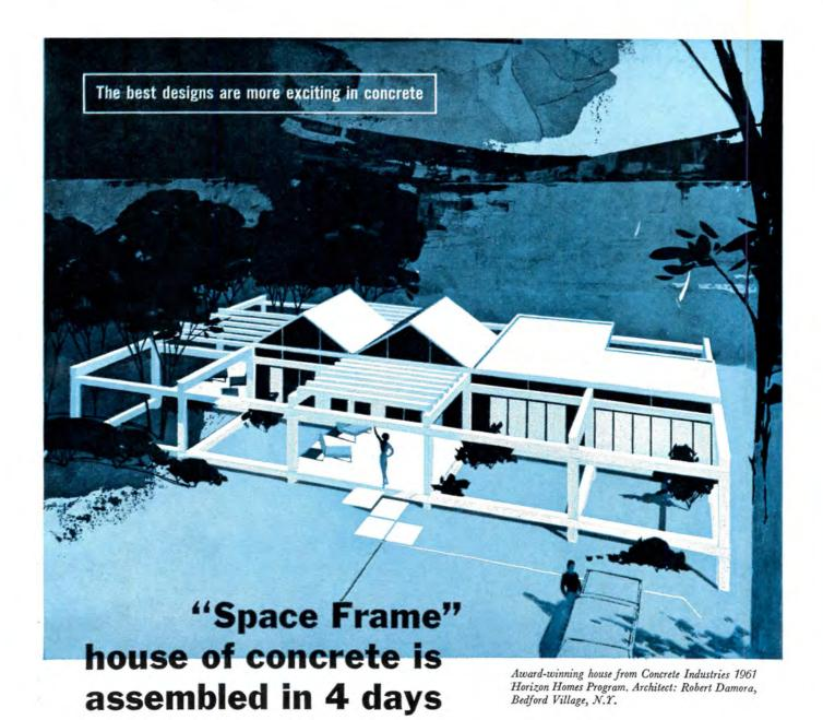
Out of the 1961 Horizon Homes Program comes this imaginative new design. The "Space Frame" house is all concrete. It is based on 16- x 16-foot modules that can be individually roofed, walled and floored. Only 6 standard sizes of precast concrete beams and panels are used.
