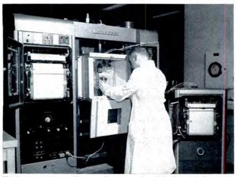
This Instron testing machine records stress-strain relationship of built-up roofing samples over a temperature range of from  $+100~\mathrm{F}$  down to a sub-zero  $-20\mathrm{F}$
