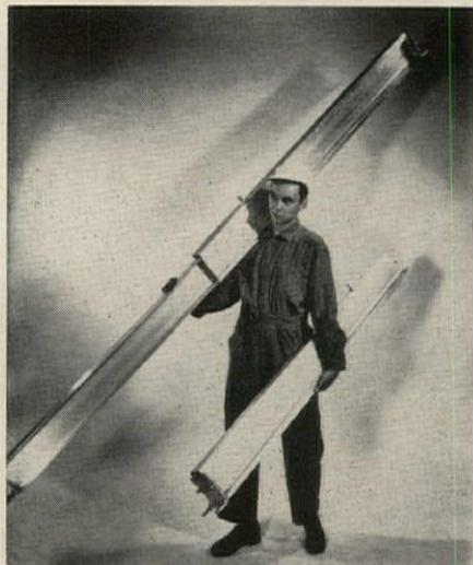
as a support for concrete slab forms for spans from 5 ft 9 in. to 9 ft 9 in. The beam has a built-in camber curve, and bending moment is 3,000 lbs, with an end reaction of 1,750 lbs. *Aluminum Co. of America, 1501 Alcoa Bldg., Pittsburgh 19, Pa.*
