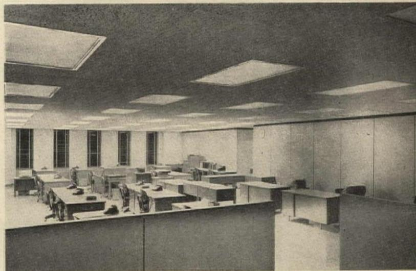
Window spacing on typical floor (shown in plan at left and photo above) is based on minimum office space requirements. Lighting levels range from 100-200 footcandles, depending on the type of work. On the 12th floor the fenestration module changes and reflects special uses. The exterior walls enclosing an auditorium on this floor are unbroken by windows, and those surrounding a lounge consist of large panels of glass divided by slender mullions
