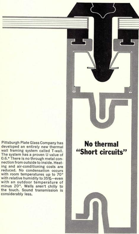
PPG T-wall is versatile. It can be glazed in combinations of %" glass, 1/4" glass, Spandrelite® panels, Twindow<sup>®</sup> Insulating Glass, insulated panels or operating sash. T-wall mullions are available in three depths: 2", 41/2" and 6", to meet various strength and design requirements.
