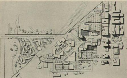
Pittsfield, Massachusetts downtown renewal plan was designed for an unspecific and changeable set of conditions. Architects developed cross axis to main street, placed tall building to terminate axis. Most of off-street parking required had to be accommodated at grade, but cars have been hidden behind buildings as much as possible.
