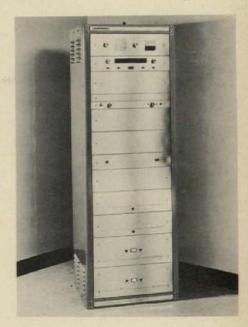
Motorola has announced the introduction of a complete line of solid state hospital music and voice paging facilities including AM/FM radio, a tape playback deck and record changer, and a variety of speaker systems. Solid-state amplifiers are available in 50 and 100 watts; all input connections are of the plug-in or screw-terminal type to facilitate installation. The transistorized AM/FM tuner has temperature compensated circuits to eliminate tuning drift. . Motorola Inc., Chicago.
