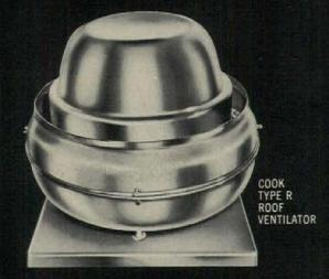
Low, compact. Blows fumes or grease-laden air high above the roof. All aluminum, including the airfoil blower wheel. Belt or direct drive, 7" to 48" wheel. Completely weatherproof construction. Insulated motor plate.
