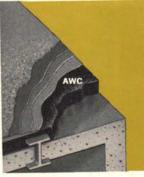
Easy removal makes AWC ideal for future floor applications. Even covers reinforcing stubs and beams.
