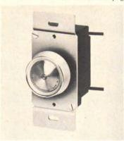
600-WATT DIMMERS / Two new UL listed solid-state incandescent dimmers, the single pole DI-61UL and the three-way DI-63 UL, carry a rating of 600 watts and feature press action on/off operaation. Each unit has only two moving parts—a switch and a long-life potentiometer. Current is controlled by a solid state switch that lasts indefinitely. Special heat dissipation techniques contribute to the long life of these devices.
