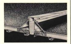
In addition to protection from cracked felts along the water dams, the expansion joint provides safeguards against leakage into the joint itself. A vinyl strip at the bottom, from one roof edge to the other, moves with the roof to form a positive, continuous seal. The extruded aluminum sides and related components, being free-floating, are also independent of thermal reaction between the water dam and felts, Transitions and junctions are factory fabricated.
