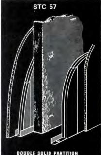
spaced 4" apart, with insulation (3" thick, 2 pcf Fiberglas® or 3" thick standard R-11 Fiberglas® or 2" thick mineral wool) stapled to the back of one core in the cavity. Over the cores, Gold Bond ½" wallboard is laminated to each side. STC is 57. (Geiger and Hamme, NG 218 Ft and NG 222 Ft and NGC Testing Lab.) Angles, shown at right, were used in sound tests. Channels are optional.
