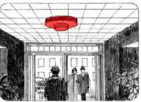
**Lobbies** Chromalox Type VUH Ceiling-Mounted Electric Vertical Unit Heaters are installed in entryways and stairwells to form a warm air barrier to cold outdoor air. Optional discharge air diffusers provide a choice of five heat distribution patterns. Larger sizes up to 50 KW are ideal for high bay mounting.
