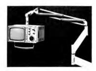
HOSPITAL TELEVISION SYSTEM / A fully transistorized electronic system provides both audio and video intercommunication in addition to furnishing individualized TV entertainment for patients. The system requires only a single coaxial wire. A balanced arm keeps the miniature set at the correct viewing position and within the patient's reach so that he can make all set adjustments without the aid of a nurse. . Bell Hospital Systems, Inc., Bridgeport, Conn.
