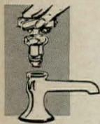
It's simple really. The faucet body doesn't wear out. The parts that do wear are all in one replaceable unit. And today's unit still fits Chicago Faucets made as much as 50 years ago—completely renews the operating heart almost as easily as you'd change a light bulb.
