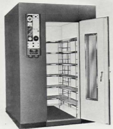
**ENVIRONMENTAL ROOMS** / An added 8-in. interior width to the V.I.P. fifty-six controlled environmental rooms provides up to 25 per cent increase in loading area, and up to 56 cubic ft of added chamber space over previous models. The "Lumen-Aire" ceiling plenum serves as a combination air-conditioning and air-flow chamber and permits uniform light transmission throughout the room. ■ Lab-Line Envroneers Inc., Melrose Park, Ill.
