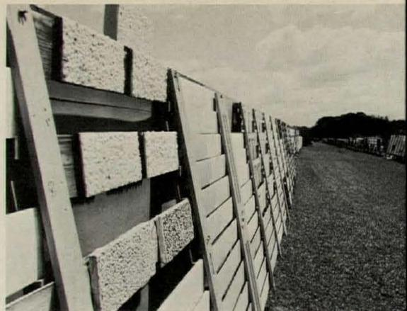
Marble chips (left) being blown into acrylic latex bedding test panels (above) show no adverse effects of weathering.
