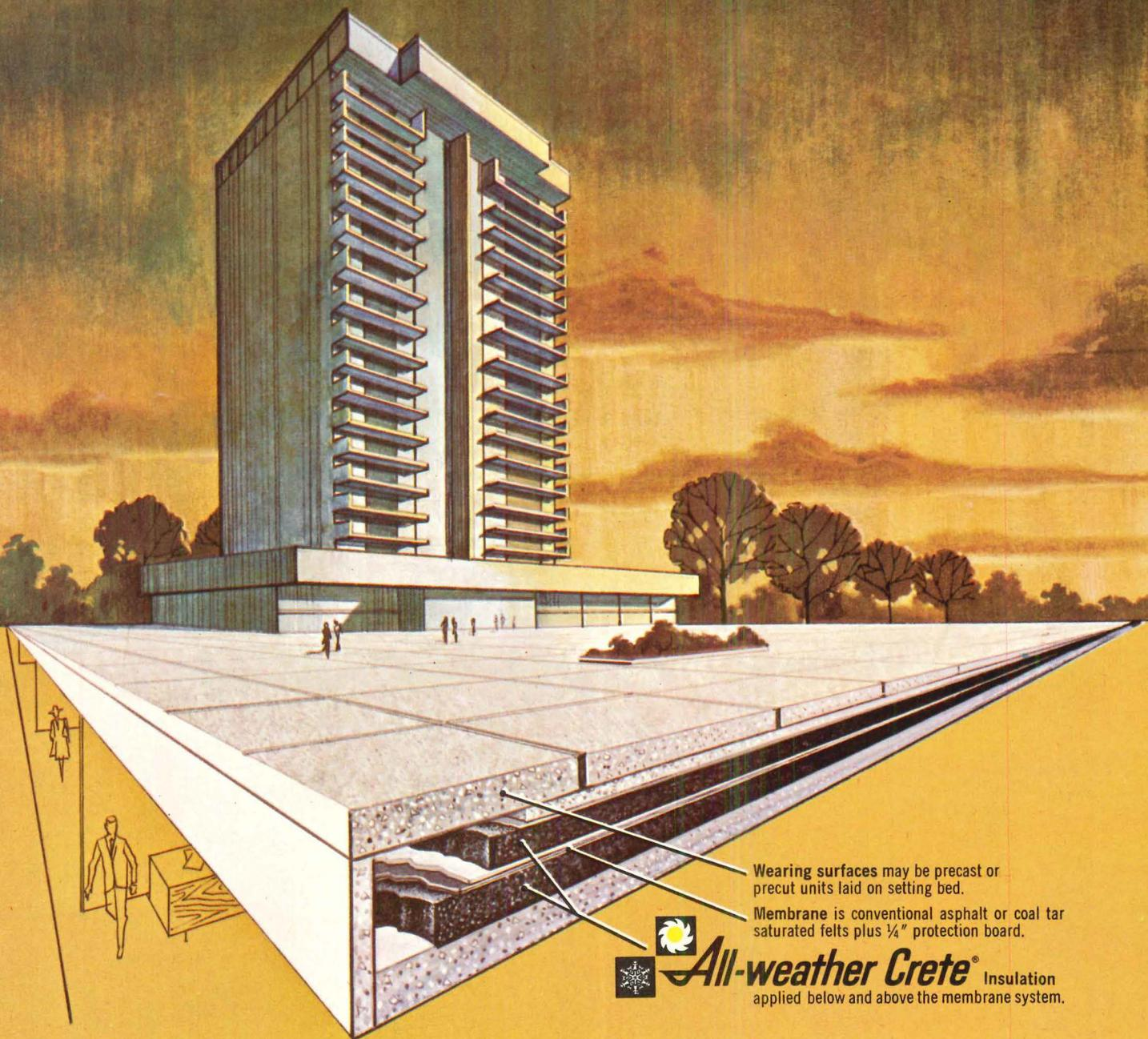
Wearing surfaces may be precast or precast units laid on setting bed.
