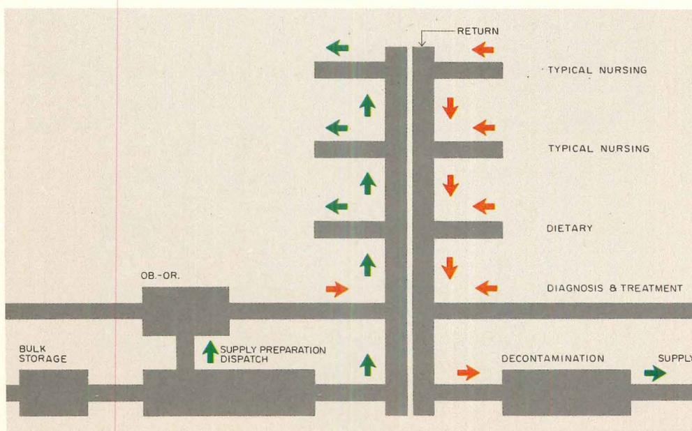
delivers new and sterilized goods to designated areas of the hospital, while the other transports garbage and soiled materials directly to the decontamination area for sorting and automatic disposal.
