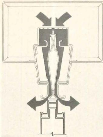
**AIR CONDITIONING** / Two streams of supply air, each under independent automatic control, are discharged in opposite directions from parallel diffuser openings of *Dual Moduline Weathermaster* units. This arrangement, plus a diffuser section only
