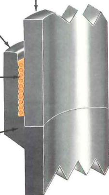
**90 SECONDS** of controlled heat—applied by the exclusive, patented GSR FUSEAL process—joins GSR FUSEAL polypropylene fittings and pipe into a leakproof, distortion-free, homogeneous unit. Add the superior chemical resistance of polypropylene and the certainty of this improved joining technique—and you have the ideal method of handling corrosive wastes.
