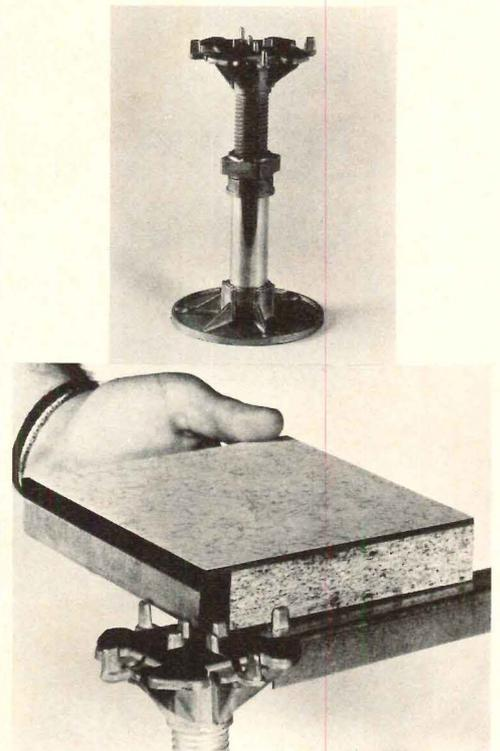
**RAISED FLOORING** / A heavy-duty aluminum pedestal and steel-encased particle-board panels are designed to increase strength and durability in raised flooring, while dampening noise transmission. The pedestal automatically locks in place at any height, and each 24-in.-sq panel will support a 1000 lb concentrated load and a 250-lb-per-sq-ft distributed load with a 4-to-1 safety margin. ■ Westinghouse Architectural Systems Department, Grand Rapids, Mich.
