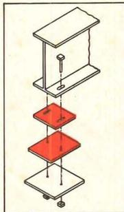
Shown at the left is the simple principle of expansion joints surfaced with TEFLON fluorocarbon resin. Two surfaces of low-friction TEFLON slide against each other, allowing free lateral movement to accommodate all thermal expansions and contractions as well as stresses due to storms.
