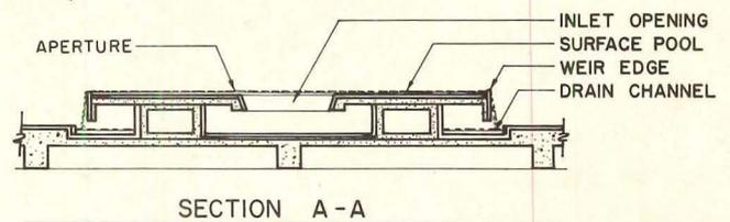
2. Draining and recirculating 5,000 to 6,000 gpm without the benefit of a retention pool. The only available depth for this was 9 to 12 in. between the sloped plaza paving and the plaza structural slab. The elevations were already set, and it was not possible to depress the structural slab.
