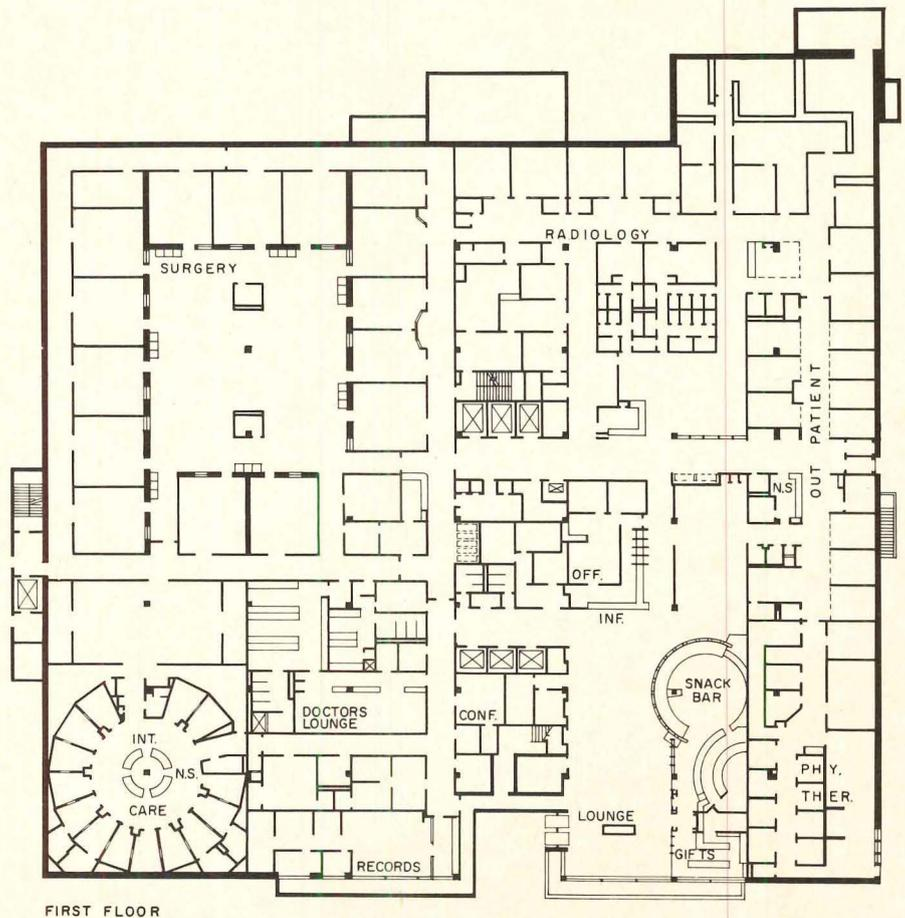
Plans below show that there is driveway access to the basement, which contains staff parking, boiler plant and pick-up rooms for trash and soiled linen. The first floor has the main entrance and emergency and employes entrances all on grade. Vertical transport systems in the hospital permit this floor to carry related departments of intensive care, surgery,
