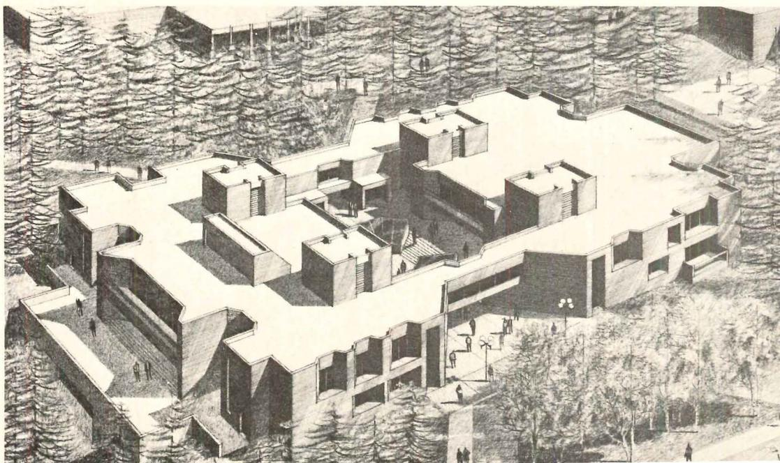
**Usdan Student Union**, Brandeis University, Waltham, Massachusetts, is designed as a compact, three-level structure of interconnecting wings around an outdoor courtyard. Paired core-towers containing stairs and elevators define the wings and emphasize the individual entrances. Windows are deeply recessed with 45 degree jamb details. Architects: Hugh Stubbins and Associates.
