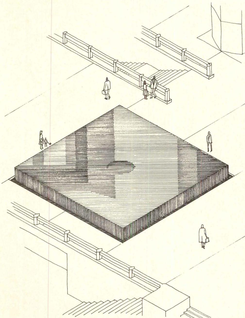
Fountain for plaza of Bank of America World Headquarters in San Francisco is a shallow pool with water falling from all four sides, forming a vertical sheet of water that "bends" the corner. Base of the pool is a 24-in.-high granite skirt.
