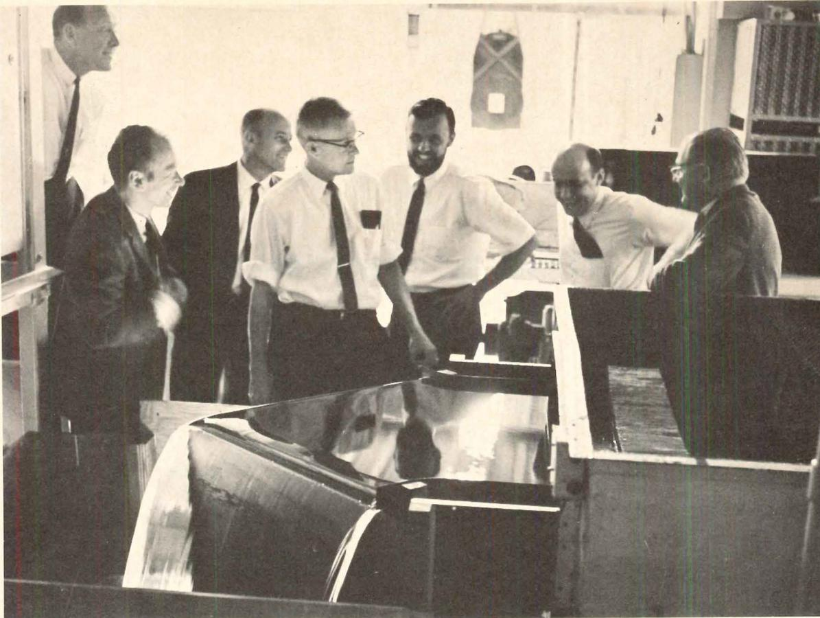
Though there was some doubt about the possibility of creating a waterfall with "square" corners, hydraulic engineers at the University of California at Berkeley accomplished the feat by curving the weir at the corner in section and elevation (see drawings of weir corner condition across page). Away from the corners the weir is a simple wedge. Several corner designs were tried—such as large radius drop, notching, spout. The final configuration (across page) was tested in a full-size corner.
