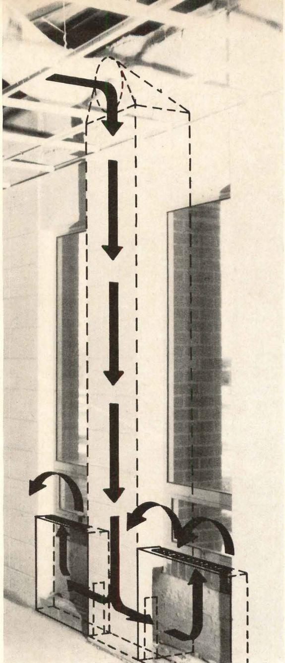
An outside design temperature of  $-25^{\circ}$  F at Watertown, South Dakota, made it desirable to have perimeter distribution of heat in the Watertown Vocational-Technical School. This was achieved by ducting some 20% of supply air down pilasters into wall ducts. Balance of air was supplied by ceiling ducts. Architects: Harold Spitznagel & Associates; Pope and Robel. Engineer: Harold Spitznagel & Associates.
