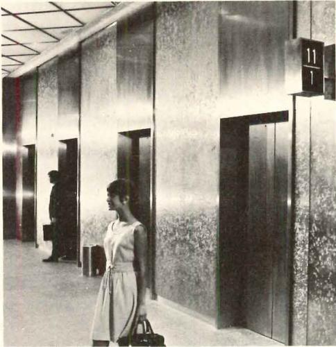
**STEEL INTERIORS** / Steel with designs recessed into the surface has been used for the lobby of One Oliver Plaza in Pittsburgh, designed by William Lescaze and Associates. The *Intaglio* (engraved) finish has a fern-like pattern that may be used with different materials and colors. ■ Allegheny Ludlum Steel Corporation, Pittsburgh.
