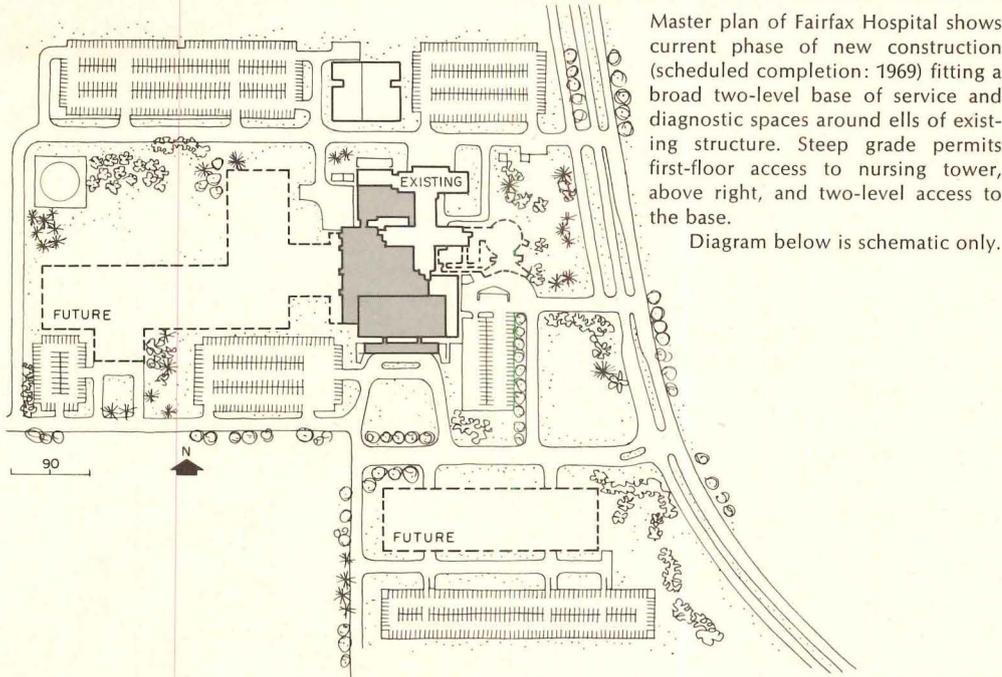
Master plan of Fairfax Hospital shows current phase of new construction (scheduled completion: 1969) fitting a broad two-level base of service and diagnostic spaces around ells of existing structure. Steep grade permits first-floor access to nursing tower, above right, and two-level access to the base.
