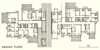
Despite height differences and plan variations among the apartment blocks of the different developers, a conscious effort has been made to develop and repeat condesign sistent elements throughout the project, such as stair towers, penthouses, and the raised roofs of banks of projecting living rooms.
