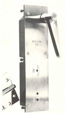
**DOOR CLOSER** / The *X-5* concealed floortype interior door closer has been "designed in response to an extensive survey of architects." It can be removed without removing the door. It can be used with stock hollow metal, aluminum or wood doors and frames with standard 4½-in. by 4½-in. butt hinges, may also be hung on offset or center pivots, and will fit in a two-in. slab. The closer is recommended for mediumtraffic interior doors weighing up to 200 lbs. ■ Rixson Inc., Franklin Park, Ill.
