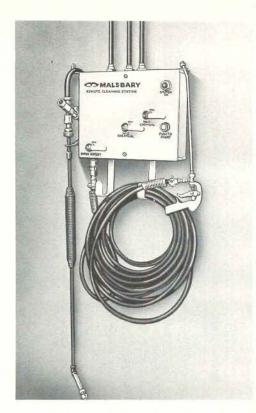
**CLEANING SYSTEM** / A system for cleaning and sanitizing food processing facilities provides a hot chemical solution under pressure and hot, clear rinse water. From a central master unit the liquids are plumbed to remote stations reaching difficult areas.
