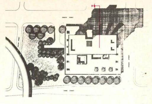
The main divisions of the building are used throughout the design to give the structure its very articulated character. Most all services are concentrated in the taller tower shaft on the building's main facade, leaving the river side free.
