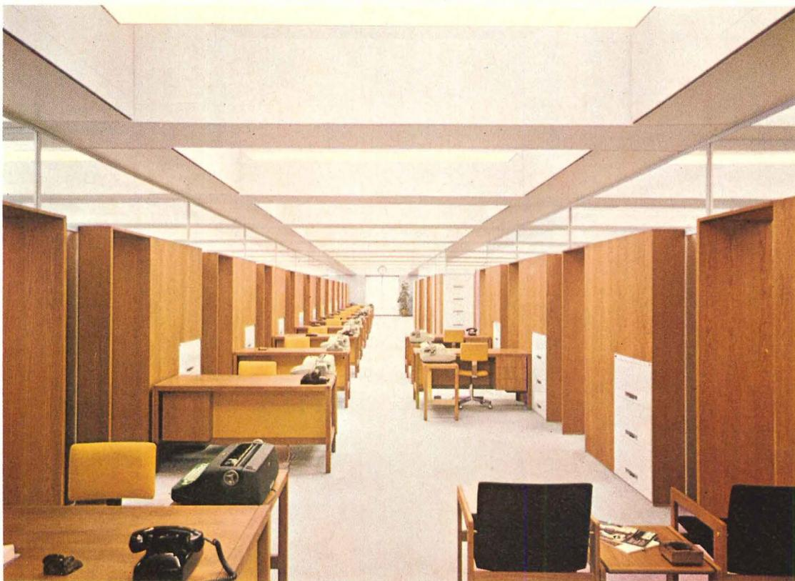
ended at a height which makes it unnoticeable beyond the second in a row; this is augmented by indirect light from each side of the ducts. One fourth the usual number of fixtures results in low-contrast, glare-free, desk-level light. Secretarial desks are designed to fit the storage wall (see section, bottom), and match it in color and wood. Floors are carpeted.
