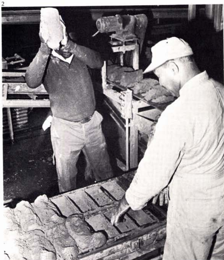
1) The pug mill where the clay is mixed and kneaded. 2) Hand-throwing into molds. 3) All handling is by conveyor belt or pallets. 4) The bricks ready for firing. 5) Finished product.
