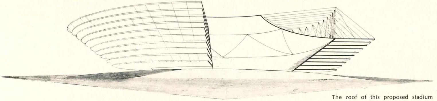
The roof of this proposed stadium design is supported by a cable structure of unusual configuration. The cables are stretched from one side of the compression ring to the other in three directions forming a criss-cross pattern. This avoids the need for a tension ring, and thus the number of cable connectors is approximately halved—an appreciable saving in cost. The weight of the roof, cables and the live load is counterbalanced by the weight of parking ramps on the exterior.
