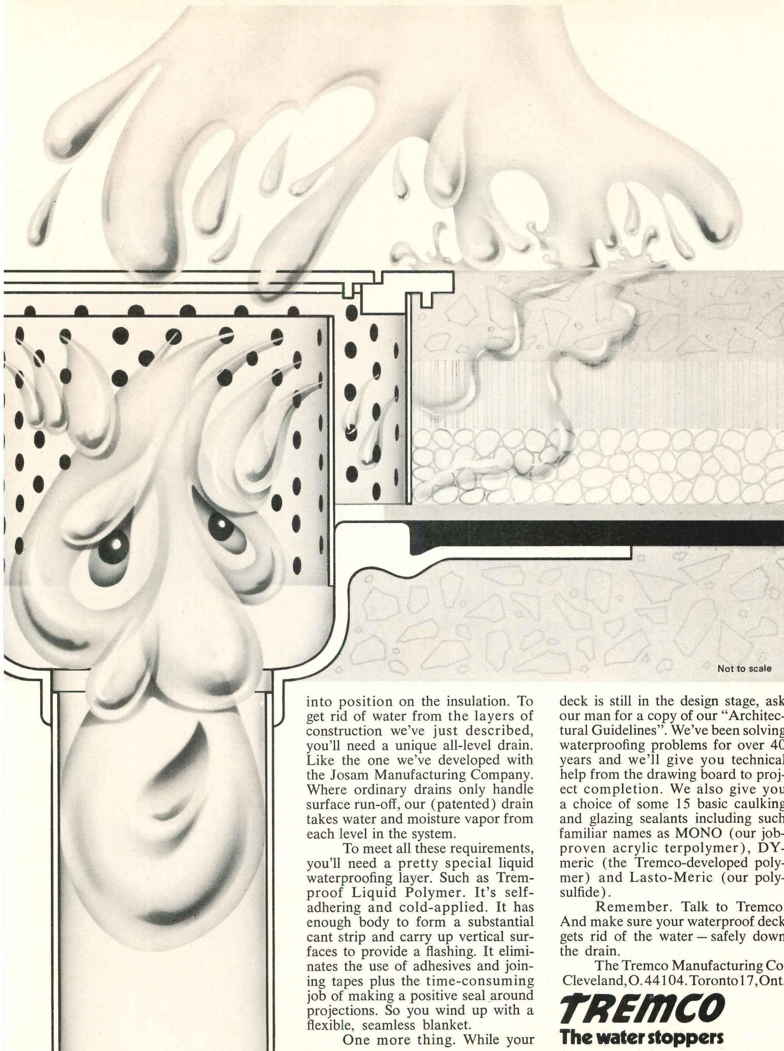
into position on the insulation. To get rid of water from the layers of construction we've just described, you'll need a unique all-level drain. Like the one we've developed with the Josam Manufacturing Company. Where ordinary drains only handle surface run-off, our (patented) drain takes water and moisture vapor from each level in the system.
