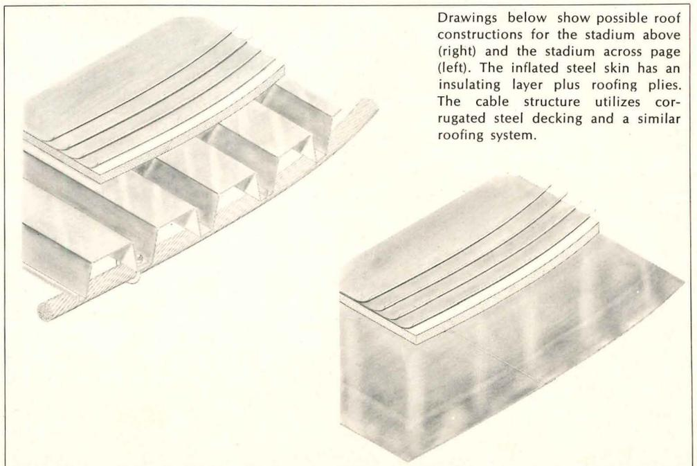
Drawings below show possible roof constructions for the stadium above (right) and the stadium across page (left). The inflated steel skin has an insulating layer plus roofing plies. The cable structure utilizes corrugated steel decking and a similar roofing system.
