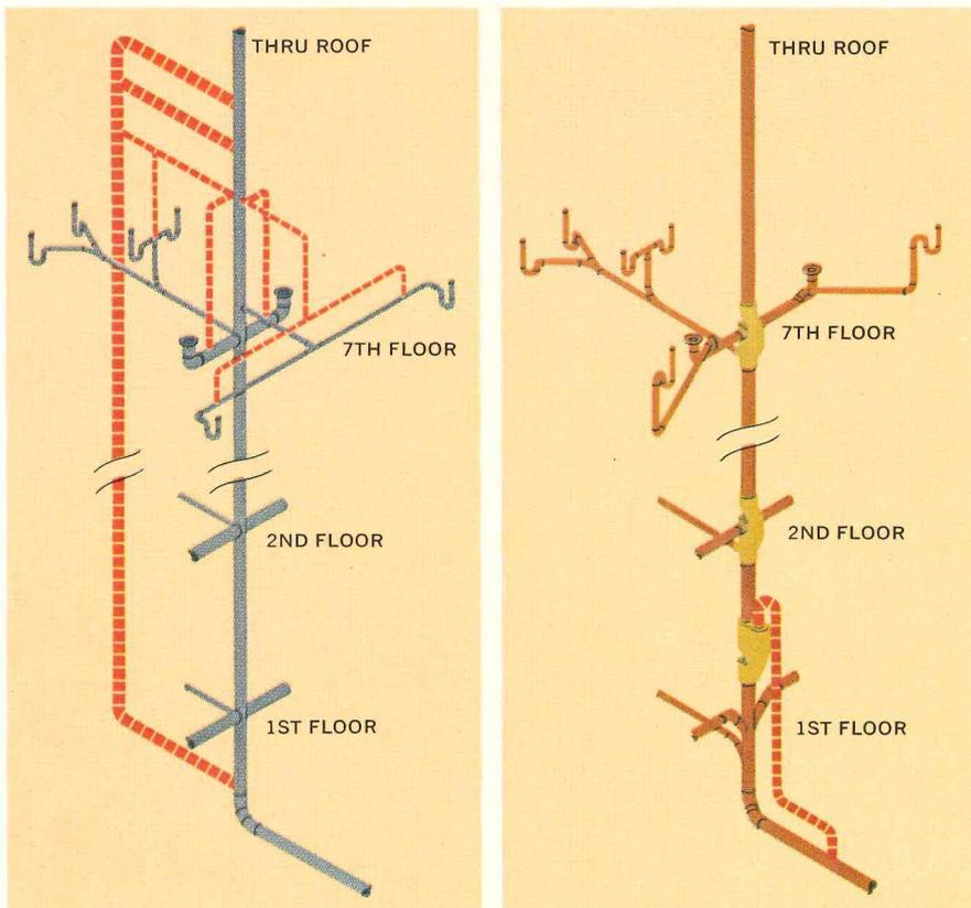
The simplicity and economy of the Copper Sovent system (right) are dramatically shown in this graphic comparison with the traditional two-pipe system. One contractor, on a recent 200-unit job, returned a credit of \$13,000 to the Housing Authority, based on savings with Sovent.
