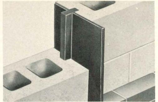
**VINYL CONTROL JOINTS** / Fillers are designed to fit standard sash blocks and provide a vertical joint for the relief of stress in concrete masonry walls. A range of sizes will accommodate 90 per cent of all masonry construction. ■ AA Wire Products Co., Chicago.
