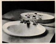
LAVATORY / The "Planet II" is a china wash basin 25-in.-wide, but shallow enough (18-in.) to fit most countertop designs. The self-rimming oval basin has twin soap recesses, concealed front overflow, and an antisplash rim. It is drilled for either 4-in. centerset or 8-in. combination fittings. It is available in marbleized china in blue, gold, green or white. . Universal-Rundle Corp., New Castle, Pa.
