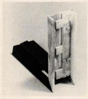
DOOR FRAME / Made of highly impact-resistant polystyrene structural foam, this molded framing system consists of two jambs and a header. Each member is made in two pieces in an expandable, interlocking arrangement to accommodate various door opening widths. Molded-in recesses take strike plate and hinges. The frames will not rot, warp, crack, split or rust. . Steves Sash & Door Co., San Antonio, Texas. Circle 316 on inquiry card
