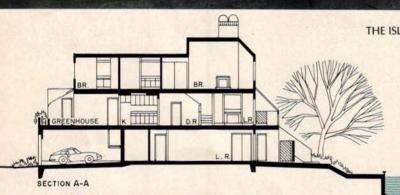
On one-third of the units, glass enclosures (often used as greenhouses) add another dimension of light to the space, and also enhance visual interest along the street. All balcony railings were constructed of tempered glass panels, providing shelter from strong winds while not obstructing views to either water or street.
