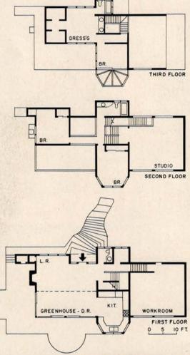
All the principal spaces in the Woerner house open through large expanses of glass to views of the marsh. The studio, photo above, is glazed using a standard industrial sash cut at its edges to fit the curvature of the roof. The plans show a simple, compact, well organized space.
