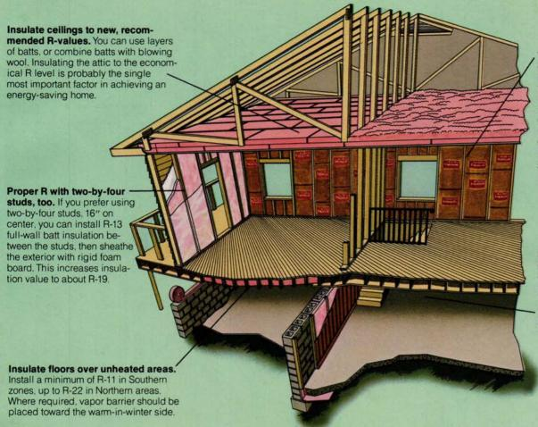
Two-by-SIX studs, 24" on center-cuts framing lumber by 30 percent! Thicker walls. to hold thicker insulation (R-19 batts), give needed strength with less lumber, often at less cost, than the usual two-by-four studs, 16" on center. Also, you can use lumber of less expensive grade, and two-by-THREE studs for interior non-loadbearing partitions.
