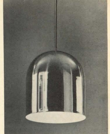
**PENDANT LIGHTING** / The "37135" pendant fixture is made of heavy gauge spun aluminum, to house a 300-watt reflector lamp. The inner surface of the shade is finished in matte white for high reflectance. The dome-shape fixture measures 12-in. in diameter by 14-in. deep, and is available in the following finishes: polished brass or chrome; matte white or black, satin bronze; and wet red. Fixture may be either cord suspended or stem mounted. ■ Habitat Inc., New York City.
