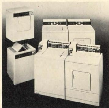
**COIN-OP LAUNDRY EQUIPMENT** / Heavy-duty commercial washers have energy-saving and security features. To cut water heating costs, a valve reduces the warm water ratio of "hot" water mixed with "cold" for both wash and rinse cycles; a "Power Miser" switch allows only cold water rinses. Money boxes are protected by high-security meter cases, and may be padlocked; the timer is also lockable. ■ Sears, Roebuck and Co., Chicago, Ill.
