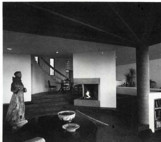
The principal interior finishes are oak strips for floors and gypsum board for walls and ceilings. Horizontal support members are either concrete or laminated wood beams.
