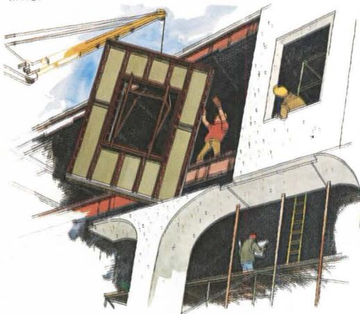
Prefabricated steel framing assemblies with exterior facing applied provide lightweight, easy to handle panels that speed curtain wall installation. Framed openings are incorporated. Curved or angled shapes are easily executed.
