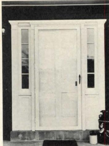
**STORM DOOR** / The "Grande Entrance" door has a 74-in.-high tempered safety glass panel which shows most of the main house door behind it. One-in. and 1½-in. thick models are available; a full screen replaces the glass panel for summer ventilation. Extruded corner gussets, spring-loaded oilite bearing hinges, and shock-absorbing U-channel vinyl glazing are door features. ■ Season-All Industries, Inc., Indiana, Pa.
