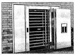
VAULT DOOR / The "Guardian" door is now available in a 7-in.-thick model, constructed of stainless steel, including the jambs, vestibule and door hinges. Security features include the Rapidial, which operates two keychanging four-tumbler combination locks; a 120-hr time lock to monitor door opening and closing; and relock devices to protect against attack with torches, explosives and drills. The door provides a clear opening 36-in. wide and 78-in. high . Diebold, Inc., Canton, Ohio.
