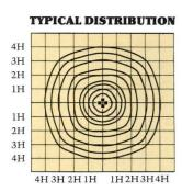
specular aluminum reflector, polished and anodized for 85% reflectance. The result is a highly efficient new distribution pattern that combines the best of both square and circle, as shown in the diagram.
