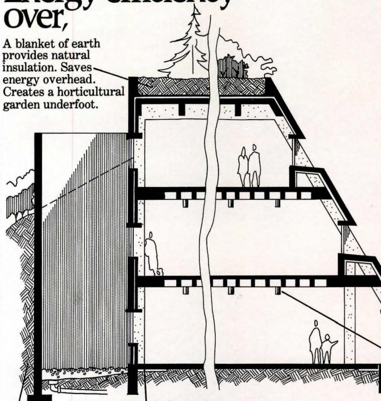
**under,** Insulation under here prevents heat loss at slab end.
