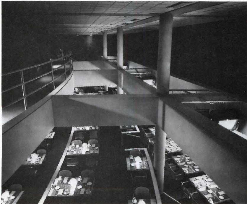
good use as a frame for unexpected diagonal vistas from the VIP level and the fast-food bar. Acoustically efficient non-asbestos mineral fibers, sprayed onto the light steel-stud walls, help to temper the echoes of cheers—and groans—as the horses enter the homestretch.
