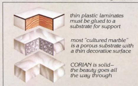
thin plastic laminates must be glued to a substrate for support
