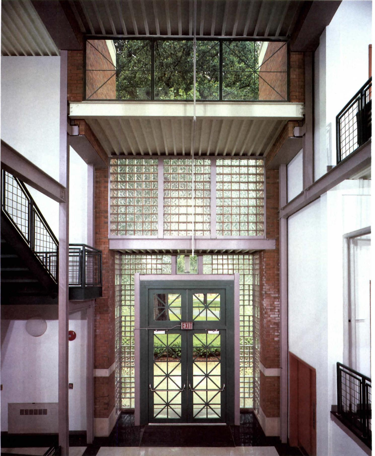
Like the exterior, the interiors of Vassar's new chemistry building derive elegance from the canny use of inelegant but wholly appropriate materials. Foremost among them is the same animating mix of glass and glass block, here combined with exposed steel and naked piping and ductwork in a medley livened by the striking use of color—grass-green columns and beams, forest-green stairs and railings, celery-green on
