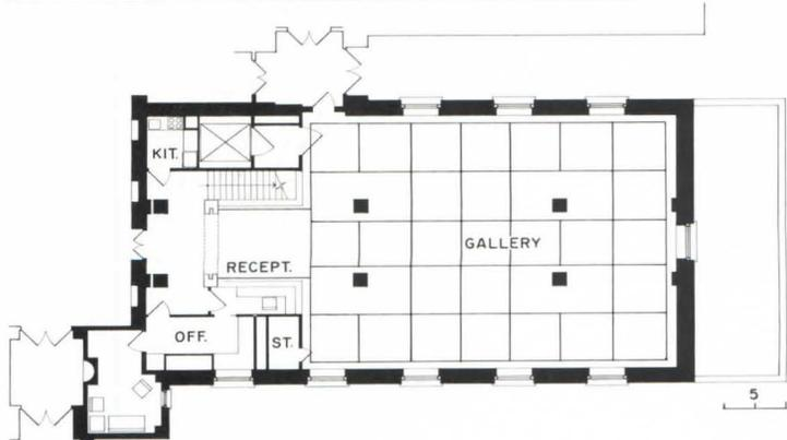
*The versatility of the floating wall system is rooted in the ease of placing its 4- by 8 1/2-foot suspended sections at any point on the nominal 8-foot grid, including the diagonal. (Recessed locking devices firmly join the sides of adjacent frames, and bases are stabilized with hidden feet like those used to level household appliances.) But its virtuosity does not end with providing almost limitlessly mutable display*
