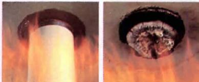
*Intumescent Fire Barrier products are the only practical UL Classified method for fire-stopping plastic pipe penetrations.*
