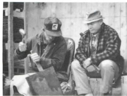
After you get the slate out of the ground, you have to break it to find the grain, and then someone like J.J. Beayon, with me in the picture, starts to split it, by hand, dividing by two over and over again. The machine hasn't been invented
