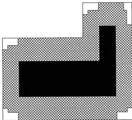
**Wind-load design for membrane roofing**
