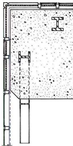
A curtainwall of anodize aluminum and reflective glass forms the skin of the Bank of China's triangulated structural frame (axonometric and photo opposite, and curtainwall detail top). Detail drawings of the curtainwall and column (above and left) illustrate the concrete connection that envelops steel members where they meet at the tower's corners.
