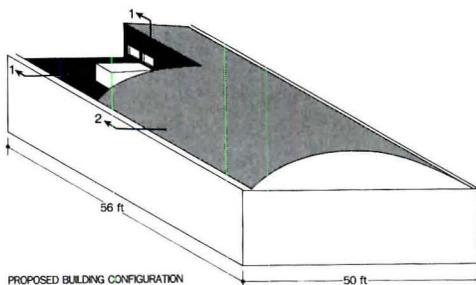
**Our barrel-roofed structure incorporated a narrow gutter (right) and a small flat roof with several closely spaced penetrations.**
