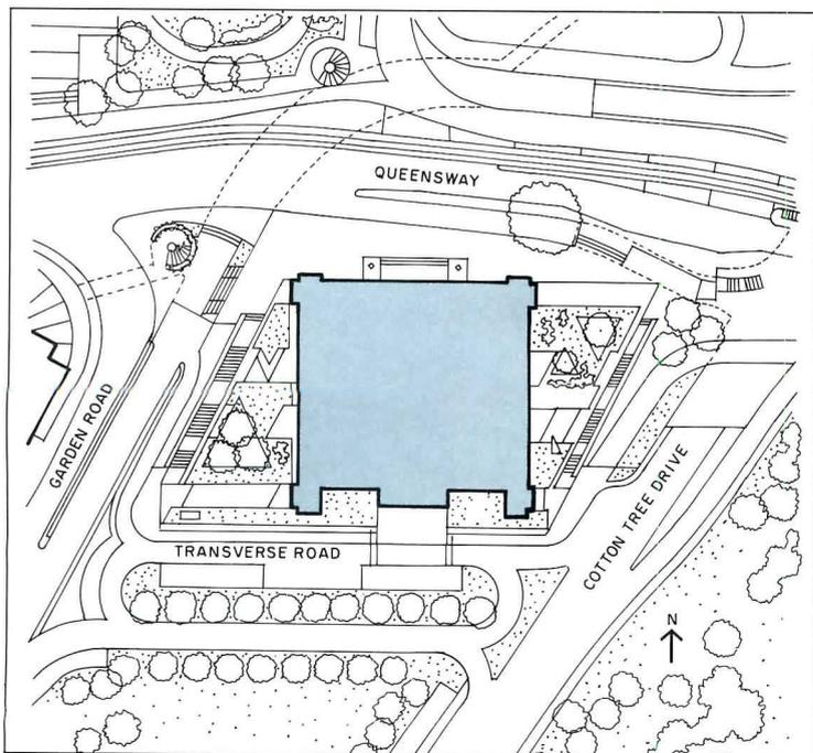
as a shaft about 165 feet square in plan. Pei divided this shaft into four triangular quadrants by crossing it with diagonals.
