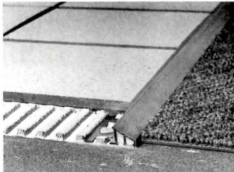
**315. Stepless transition.** The Reno-Pro file provides a sloped surface that smoothly connects tile or stone floors with floor surfaces of lower height, such as carpeting. The strip has an end leg with an inclined aluminum or brass edge attached and a perforated anchoring leg which is embedded in the tile adhesive. Different sizes accommodate tiles of four thicknesses from 5/16- to 5/8-in. Schluter Systems, Inc.
