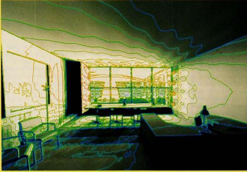
To avoid mechanically heating or cooling the concourse of the Munich Airport Center (opposite top), the engineers analyzed daylight and ambient wind and temperatures, including the contribution of surrounding buildings (opposite bottom). The fabric and glass concourse roof (left) is supported by "banana"
