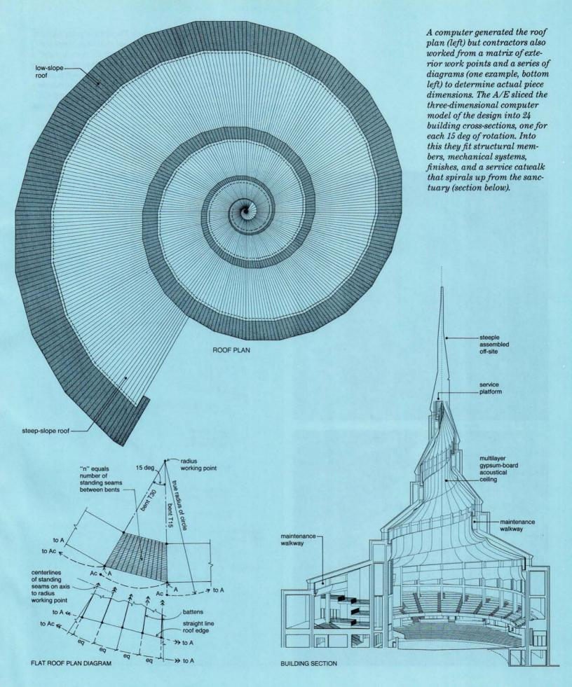
CAD software developed a three-dimensional external shell, locating points (instead of dimensions, all of which vary) at any position on the exterior (top drawing). From the shell the design team worked inward, accounting for the depth of roofing, insulation, and metal deck, thereby defining the envelope within which the structural supports were positioned (bottom draw-
