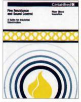
New 12-page brochure offers architects data on the sound control and fire resistance properties of fiber glass insulation. Explains terminology, details existing codes and states standard measurement procedures. Also contains detailed drawings of more common wall assemblies for buildings.
