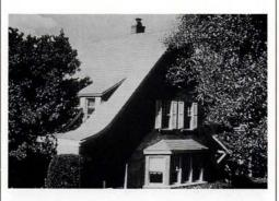
**344.** Reroof option. The Homecrest aluminum shingle, a new style, has an authentic slate, shingle, or tile texture, offered in five colors. The lightweight, individually fastened pieces are installed from the ridge down. Alcoa Building Products, Sidney, Ohio. ■
