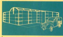
In 1973, the author proposed converting pressed-metal body parts from the Citroen 2cv into an emergency housing system for Chile. Van body parts form siding and a roof. The windshield and cab (2) provide clerestory lighting and ventilation. The prototype (3) was designed by Jeff Skorneck. (Similarly, a Dutch architect's 1975 office building used welded oil drums, camper-van roof panels, and glass bottles.)
