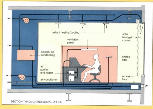
Kajima's research and development arm has preposed workspaces that include individual control of temperature, air quality, and ventilation.
