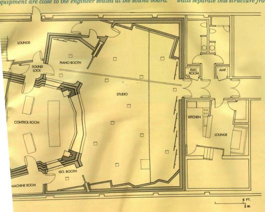
In the studio, "you want a small controlled space, but you also want as much [spatial] volume as possible," explains Peter Gruneisen. A multilayer stud-wall construction isolates the recording and control areas from exterior noise (left). The number and kinds of layers vary according to location. The studio is set on an isolating slab (sections opposite).
