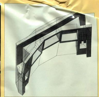
A concrete frame contains both audio and video monitors. Stud walls separate this structure from the recording studio.
