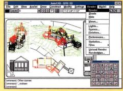
A multiple-view drawing in AutoCAD for Windows Release 12 features a deep pulldown menu to activate rendering, floating toolbox (lower right corner), and AutoCAD command line (lower left). Part of toolbar is visible beneath render menu.
