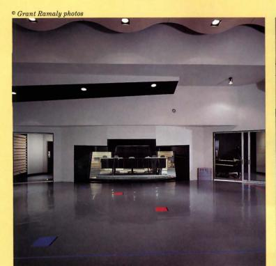
Canted and sloped shapes diffuse sound and prevent unwanted flutter echoes within the main studio.
