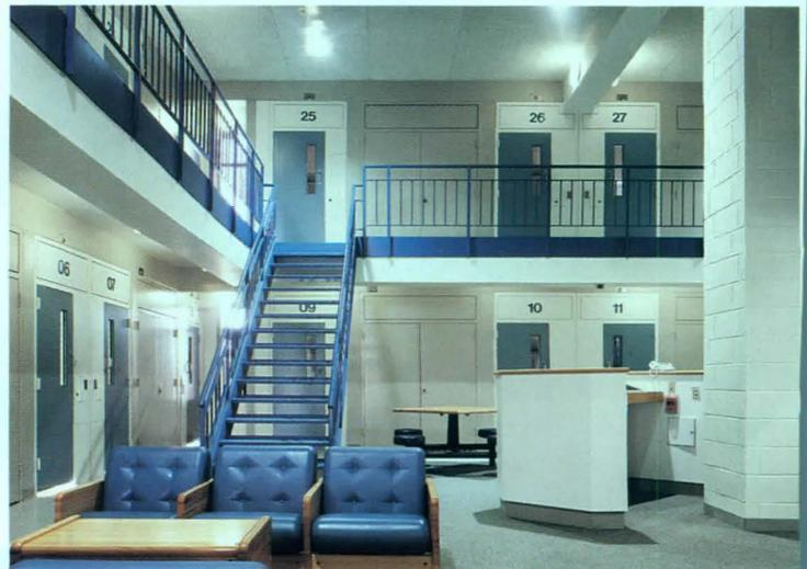
Grouped around communal day rooms (plans below and opposite) are individual cells set 20 feet above grade. The cells are 16 feet by 16 feet or 16 feet by 20 feet. Windows are in pairs vertically and horizontally to create "a public scale." An 11-story tower accommodates intake, special observation, disciplinary detention, substance-abuse treatment, and protective-
